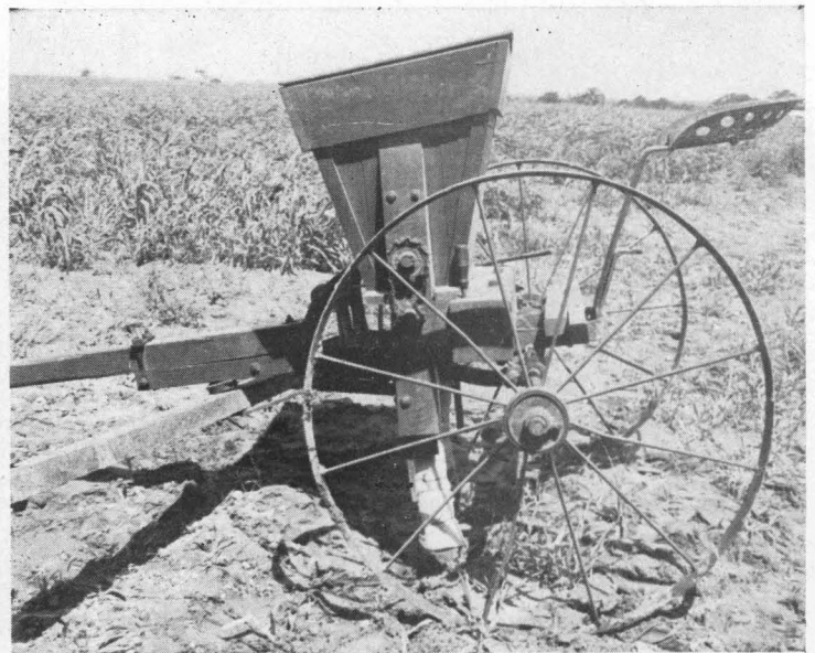
Fig. 4. View of distributor showing agitator drive.
