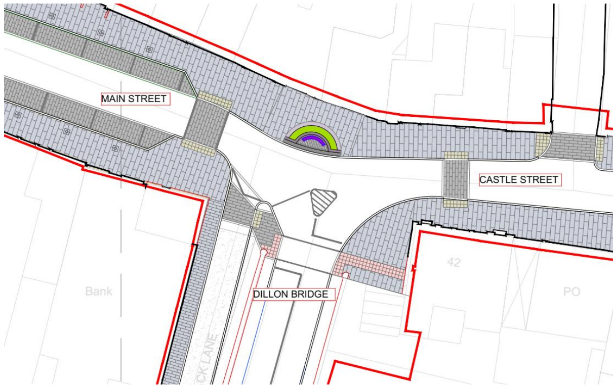
Figure 5.1: Proposed priority junction layout at Main Street / Castle Street / Dillon Bridge
