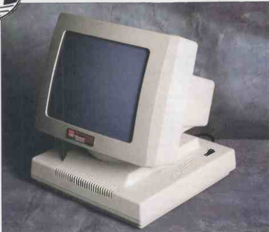
The monitor is terminal-dependent, but is normally 24 lines x 80 characters
