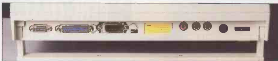
The rear ports include a non-standard MSX printer port
