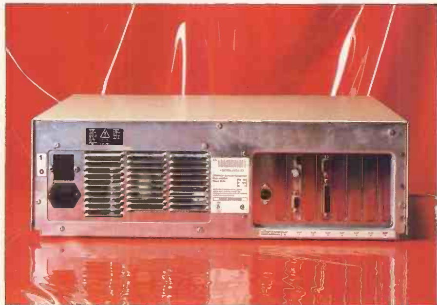
The Compaq rear panel has a power supply socket for the Compaq monitor
