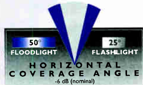
Floodlight delivers a 50° horizontal coverage pattern.
