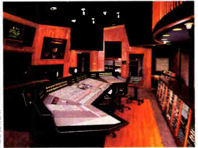
Paisley Park, Chanhassen, Minn. This famous facility's Studio A was redesigned by Glen Phoenix of Westlake Audio. Its extensive equipment list includes an SSL 8088 G Plus console with Ultimotion, a Westlake HR-1 four-way monitor system, and Yamaha and Auratone reference monitors.
