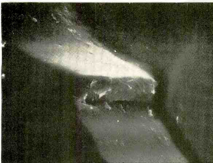
Fig. 5. Dry lubricants are trapped under the crest of an unplayable signal transient (10,000 \times ).
