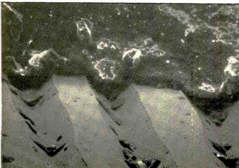
Fig. 7. “Sticky-roller” cleaner does not reach deep enough to clean groove bottoms (1,000×).
