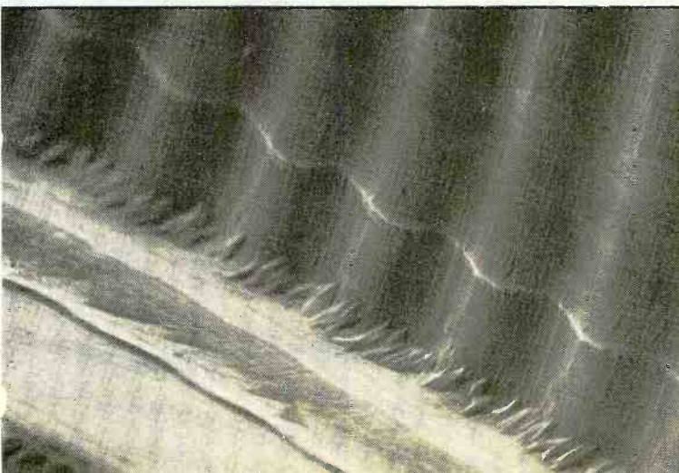
Fig. 9. Damaged groove surfaces and piled-up dirt globules in a wet-played groove (10,000 \times ).
