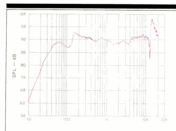
Fig. 3—One-meter, onaxis anechoic frequency response, for an input of 1 watt into 4 ohms (2.0 V).
