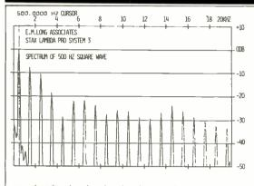
Fig. 4—Spectrum of the 500-Hz square wave as reproduced by the Stax headphones. The output is a little high at 2.5 kHz, low at 4.5 kHz, and high above 13.5 kHz.
