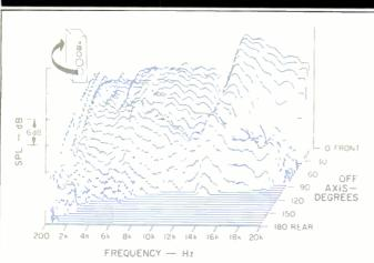
Fig. 6—Horizontal off-axis frequency responses, taken from the front, around the side, and to the rear of the speaker.
