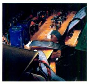
While most manufacturers use Integrated Circuits to save money. Onkyo uses costlier power transistors, resistors and capacitors because of their better performance characteristics.
