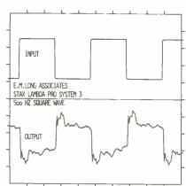
Fig. 2—A 500-Hz square wave and its reproduction by the Stax SR-Lambda Pro headphones. The output is reasonably good, especially for earphones.
