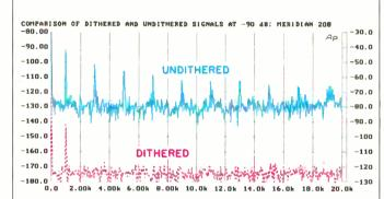
Fig. 6—Spectrum analysis of 1-kHz signals at -90 dB recorded level. Use left-hand scale for upper curve, right-hand scale for lower curve.
