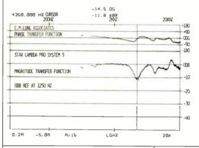
Fig. 6-Phase and amplitude spectra produced by the SR-Lambda Pro for the 30-kHz cosine pulse shown in Fig. 5. This and other curves are meant as relative measurements only, for comparison with curves in future reports. They are not meant as absolute measurements; see text.
