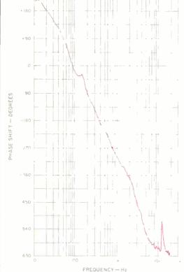
Fig. 4—One-meter, onaxis anechoic phase response.
