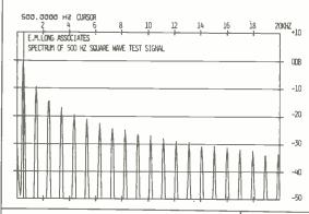
Fig. 3—Spectrum of the 500-Hz square wave shown in Fig. 2, for reference use. The harmonics are spaced at 1-kHz intervals across the spectrum.
