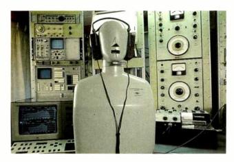
Fig. 5—Brüel & Kjaer Head and Torso Simulator (HATS), with headphones in place.
