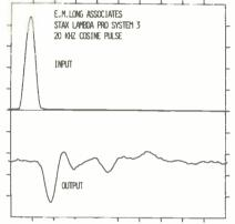
Fig. 5-A 30-kHz cosine pulse and its reproduction by the SR-Lambda Pro. Note the inverted polarity.
