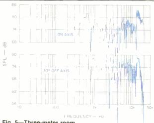
Fig. 5—Three-meter room response, on axis and 30° off horizontal axis.
