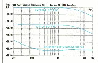
Fig. 5—Effect of input balance settings on surround outputs when feeding a mono signal to the main inputs; see text.
