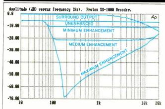
Fig. 6—Effect of Separation Enhancement circuit on main-channel outputs for input signals of opposite polarity; see text.
