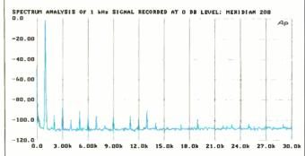
Fig. 4—Spectrum analysis of 1-kHz signal at 0 dB recorded level.
