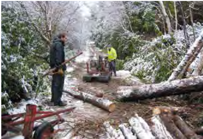
Iron Horse with powered winch but without jib or trailer being used to skid logs out of forest. Photo : anon
