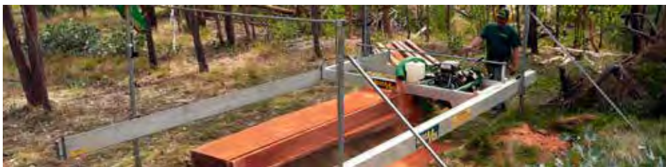
Lucas mill walked into and working in the forest.
