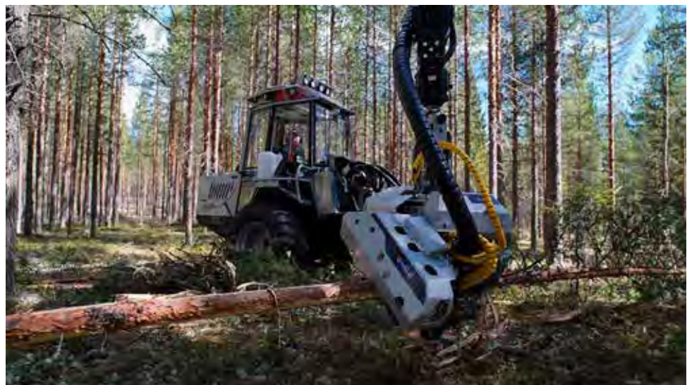
Selective thinning by mechanical harvester to create uniform shelterwood with natural regeneration of Scots pine
