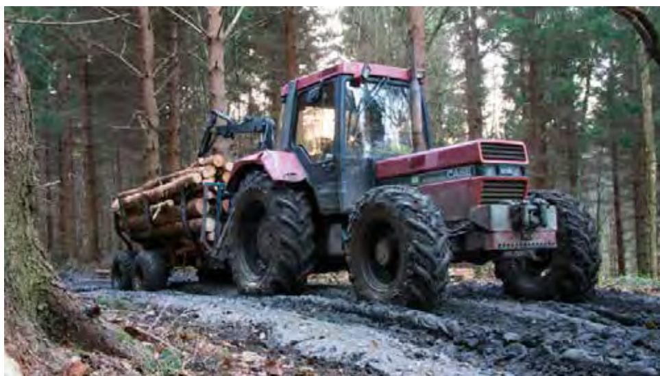
Thinning Scots pine: forwarding by 4WD tractor with trailer and jib.
