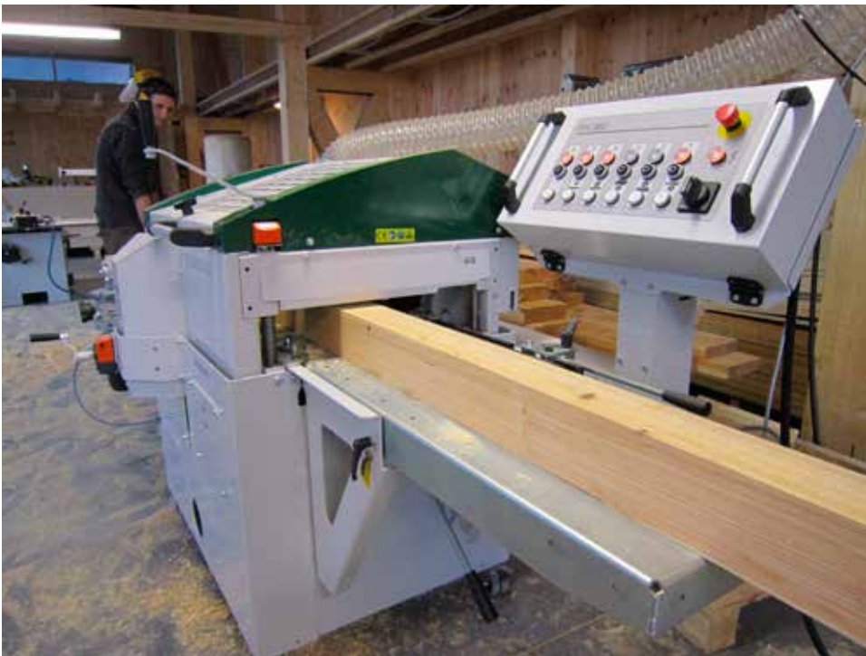
Medium scale 4-sided planer-thicknesser processing home-grown larch into structural posts and beams in a Highland workshop.
