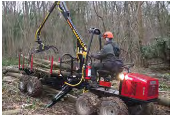
Alstor 8 x 8 with powered trailer and jib
