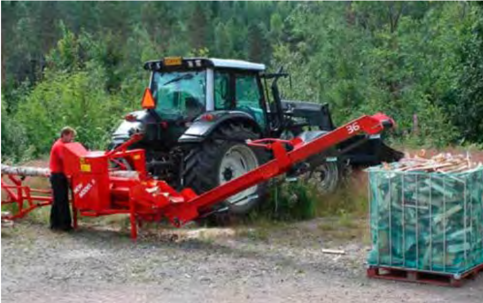
Tractor PTO powered firewood processor
