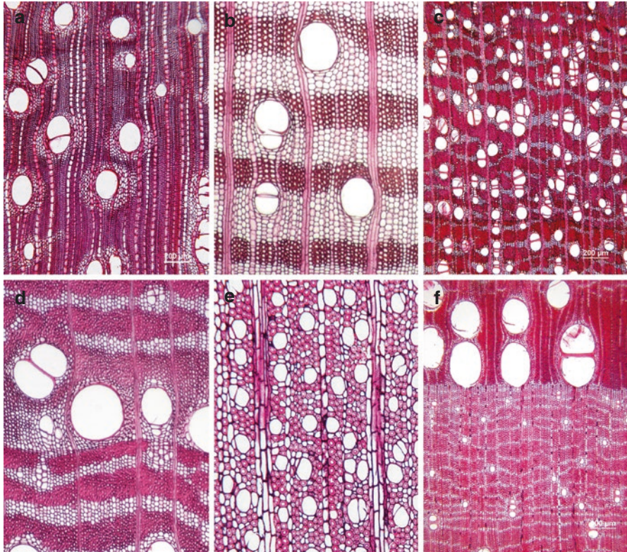
Fig. 7 Transverse sections of angiosperm woods showing a range of axial parenchyma distribution patterns. Parenchyma may ensheath vessels in wide (a) or thin layers (c, f), form tangential bands of varying width and position (b–d, f), or appear in diffuse clusters of one to several cells (e). Parenchyma cells are thin-walled and appear light in color against a background of thicker-walled fibers and vessels. Species shown are (a) Anacardium occidentale [Sapindales/Anacardiaceae], (b) Ficus maxima [Rosales/Moraceae], (c) Celtis ehrenbergiana [Rosales/Cannabaceae], (d) Sapindus mukorossi [Sapindales/Sapindaceae], (e) Viburnum stellatomentosum [Dipsacales/Adoxaceae], (f) Carya ovata var. australis [Fagales/Juglandaceae] (All images courtesy of InsideWood ( http://insidewood.lib.ncsu.edu/ ) and reproduced with permission of the original contributors (Wheeler 2011). Photo credits and copyright: (a, c, e, f) ©Elisabeth Wheeler, North Carolina State University, Raleigh, N.C., USA; (b, d) ©Els Bakker, Naturalis, Leiden, Netherlands)
