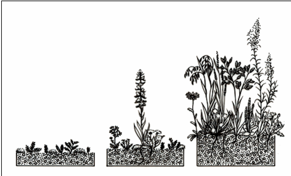
Figure 3: Different substrate depths (6, 12, and 20 cm) used to create various vegetation forms as a basis for the colonization of diverse fauna on the Cantonal Hospital roof.
