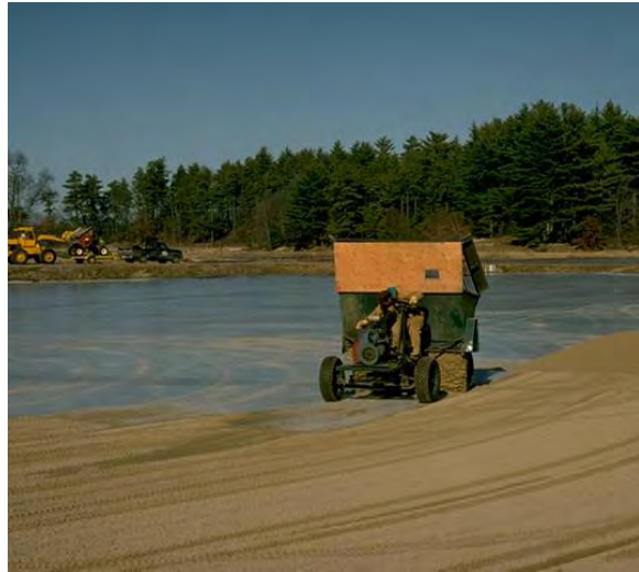
Fig. 2. Ice sanding on frozen flood waters with a sand buggy. Photo courtesy H. Sandler.
