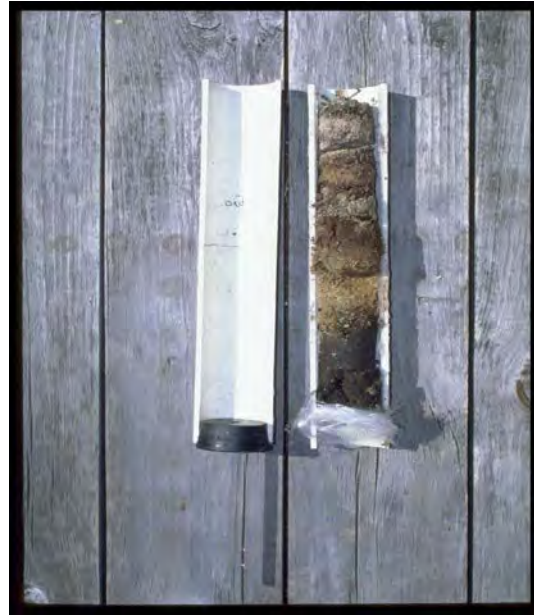
Fig. 1. Soil core profile the alternating layers of sand and organic matter found in many cranberry farms. Photo courtesy J. Davenport.
