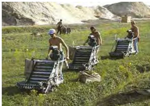
Fig. 2. Examples of self-propelled dry harvesters used to pick cranberry fruit. Photo courtesy www.FAO.com.
