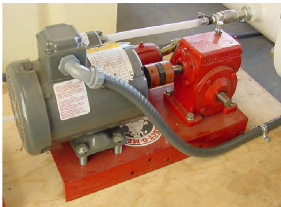
Fig. 2. (Top) Irrigation line check valve, vacuum relief valve, and low pressure drain. (Bottom) Pesticide metering pump. Diagram and photos courtesy http://www.cdpr.ca.gov/docs/emon/grndwtr/chem/chemdevices.htm .
