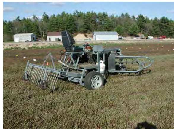
Fig. 4. Grower-manufactured pruner with knives attached to a rotating head in front combined with a hydraulic rake attachment in the rear. Photo courtesy H. Sandler.
