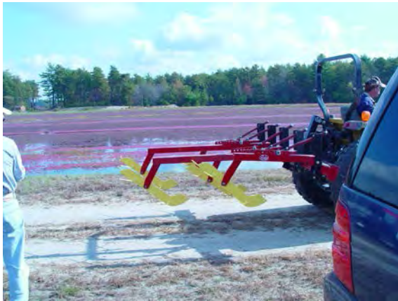
Fig. 5. Wet harvester design called the Ruby Slipper, which is rear-mounted. Note the yellow paddles instead of the metal reel seen above. Photo courtesy B. Wick.
