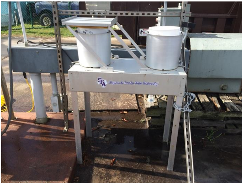
Image of the Precipitation Collector used to quantify the annual aerial \text{Na}^+ deposition at the Moody Gardens study site.
