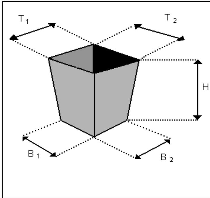
Calculate top (Y) and bottom (Z) area in square inches using T<sub>1</sub>, T<sub>2</sub>, B<sub>1</sub>, and B<sub>2</sub> in inches:
