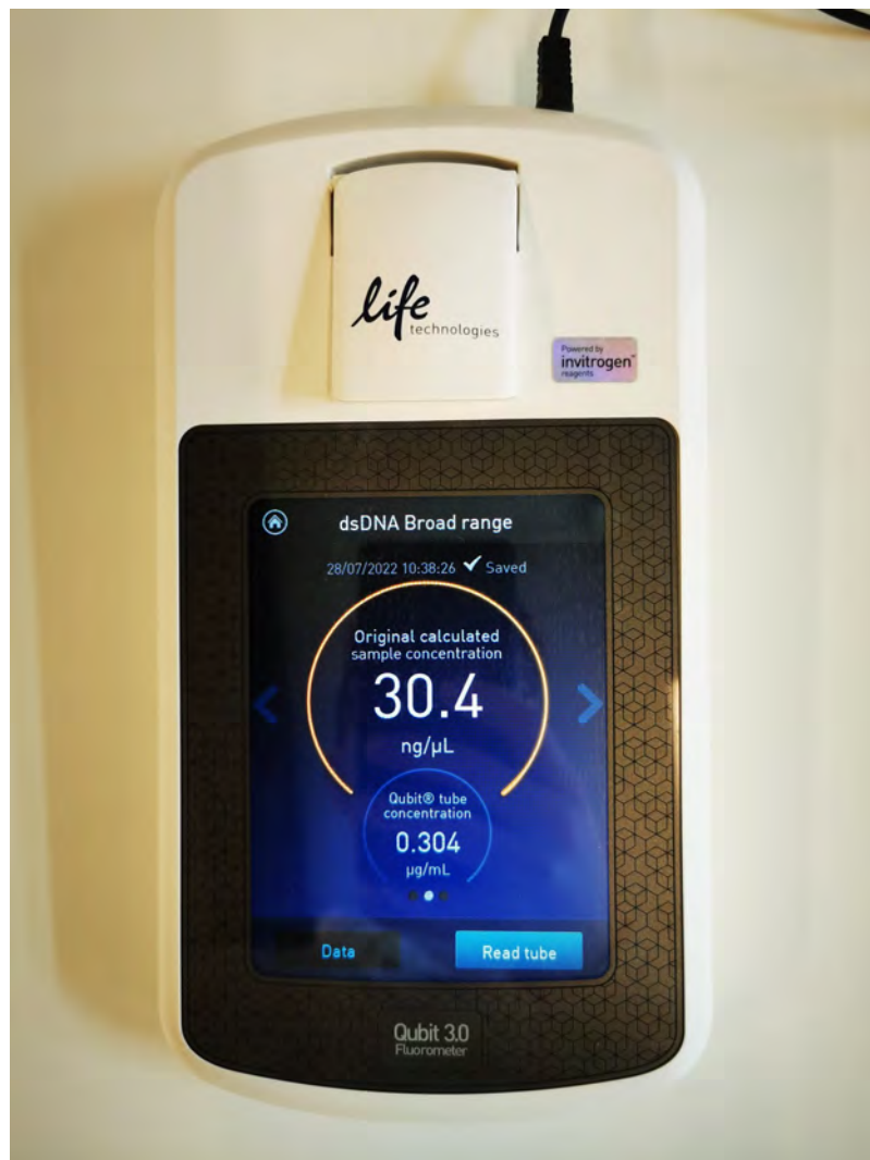
Qubit Fluorometer measuring sample DNA of B. cyanea at 30.4ng/ml
