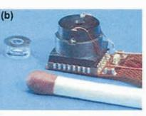
FIG. 3. (Color) (a) Optical design of the camera module containing a liquid lens; (b) the assembled camera module and the liquid lens.
