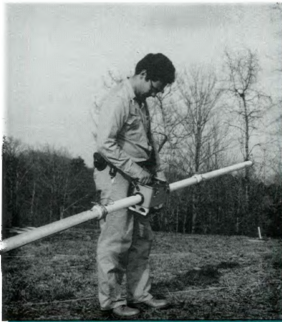
A member of a survey team measures subsurface conductivity to locate buried metal waste drums.
