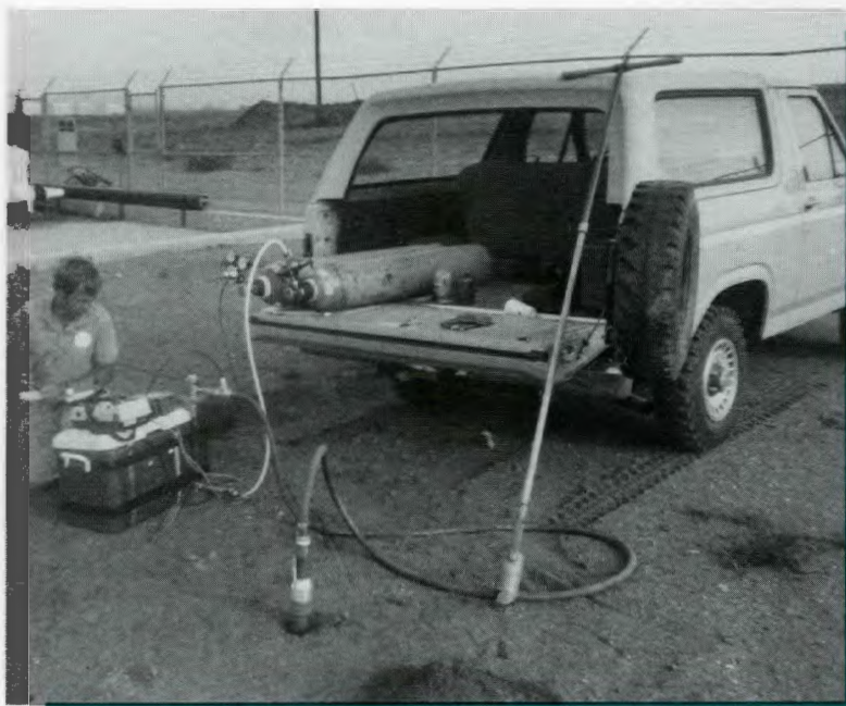
Kip Solomon measures conductivity of vapors through the soil at the Hill Air Force Base in Utah.
