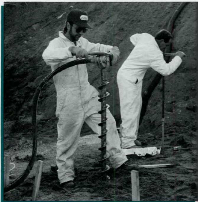
Subsurface drilling is sometimes required for sample collection, as at this jet fuel spill site.
