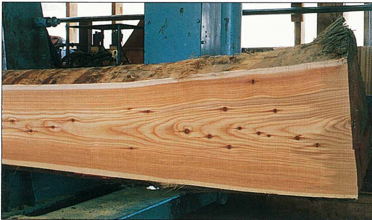
Fig. 15 - Centre sawn log of European larch (75 yr). Note narrow sapwood band, coloured heartwood, small knots, and prominent grain.
