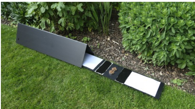
Fig. 1. Hedgehog tunnel, opened to reveal bait, ink pads and paper. Photo: Peter Sykes.
