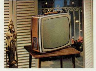
Motorola introduced and marketed in 1960 the first large-screen,transistorized portable TV, the 19P1. It operates both indoors and outdoors on regular house current or on a self-contained energy cell.
