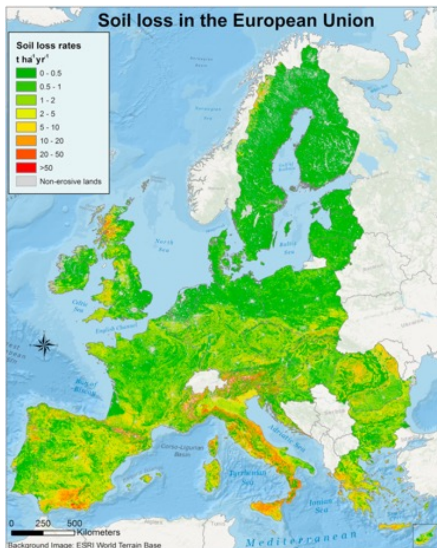
Figure 1: Map of soil loss rates in the European Union (reference year: 2010) based on RUSLE2015. Source: Panagos et al, 2015.
