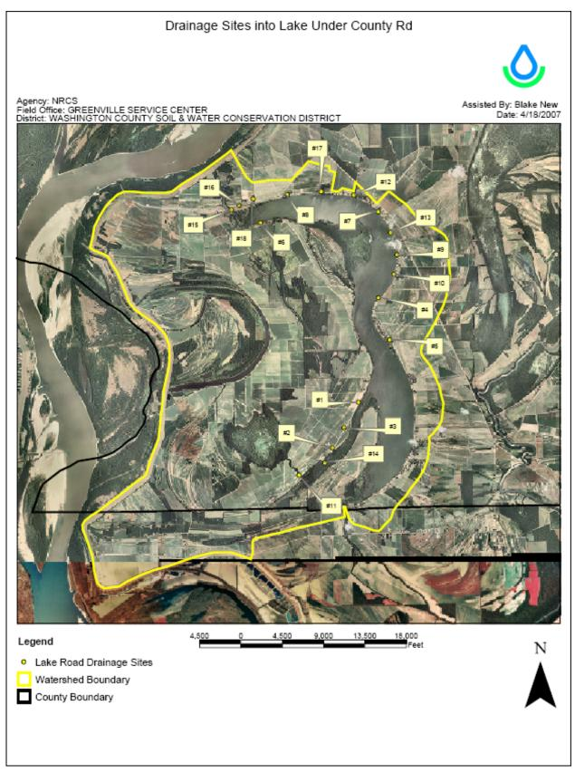
Figure 5.1. Locations of county road culverts exhibiting head-cutting.
