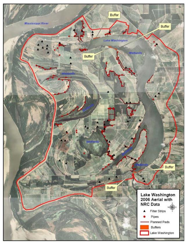
Figure 5.2. Location for sediment and nutrient BMPs.
