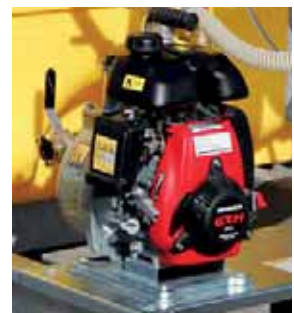
Motorpumpe HONDA 130l/min
