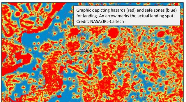
The spacecraft was equipped with two new technologies (Range Trigger and Terrain Relative Navigation) for landing the 2,263-pound (1,026-kg) rover on a hazard-free spot on the crater floor. Perseverance landed about 1.1 miles (1.7 km) from the center of the targeted area. The site is level and free from any large boulders or other obstacles with the rover reporting only a  $1.2^{\circ}$  tilt.
