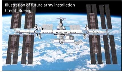
The batteries, charged by the solar arrays, provide station power when the arrays are in Earth's shadow, which occurs 16 times each day – each time for approximately 45 minutes.
