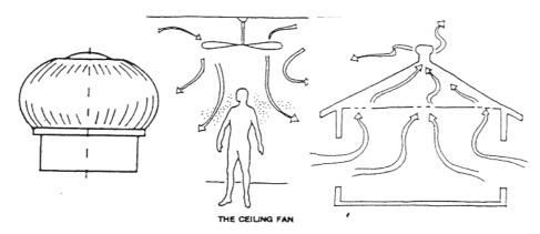
Figure 6 - Illustrating Space Cooling System.
