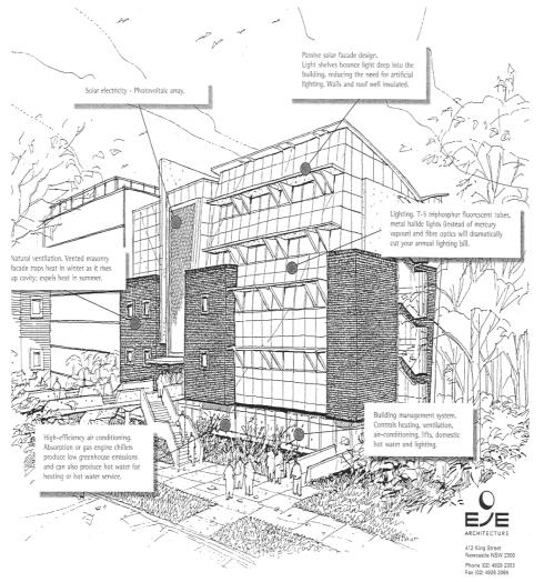
Figure 7 - Key Components of an energy efficient commercial building
