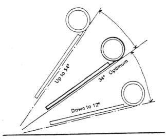
Figure 5 - Optimum range and elevation for solar collector.
