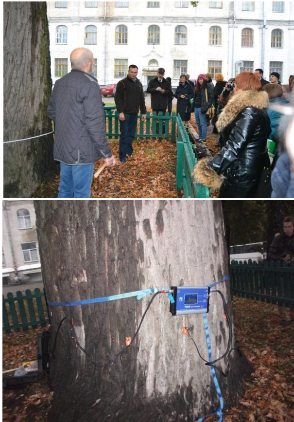
Fig. 6. Assessment of memorable trees on the territory of NULES by Tomograph PICUS 3
