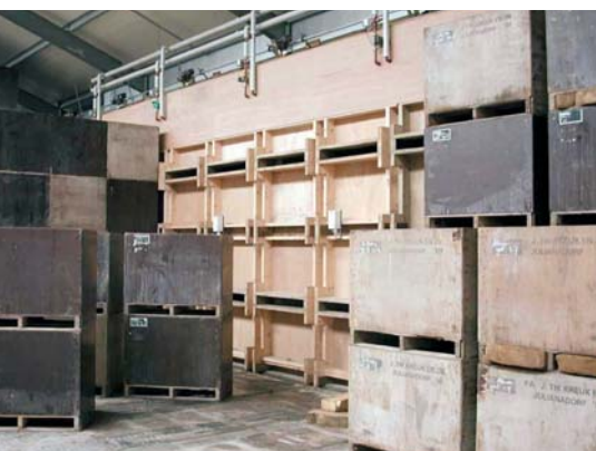
● Airwalls, a common sight in the world bulb industry. They are used to dry bulbs after lifting and to actively ventilate tulips to remove ethylene in case of Fusarium infection.
