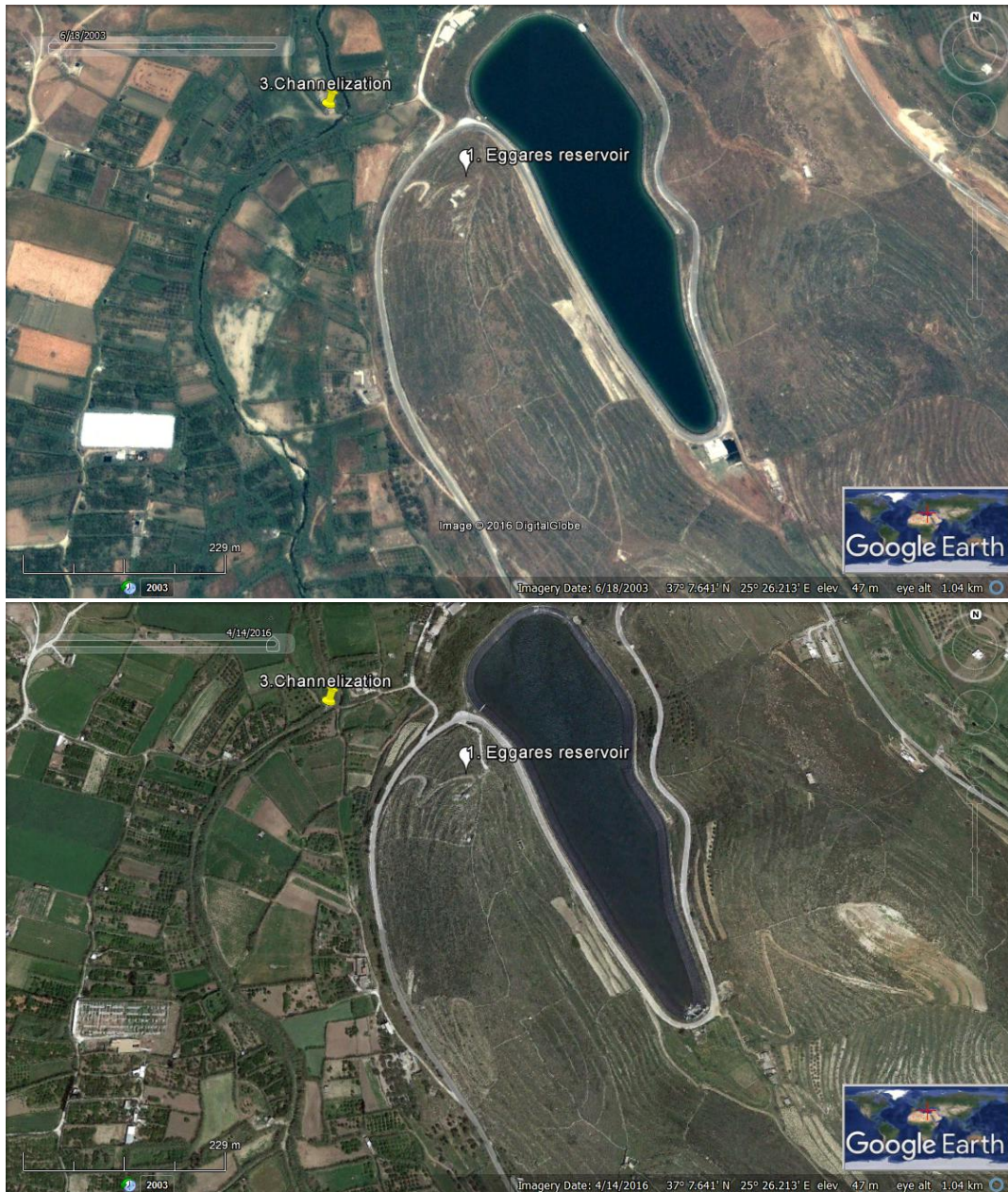
Fig. 34: Top image: 2003 – Narrowed channel but some dynamics in certain sections, water visible. Establish relationship with the weir upstream enables water flow, maintaining some dynamics. Bottom image: 2016 – Less fluvial dynamics, vegetation encroachment due to upstream regulation (weir).
