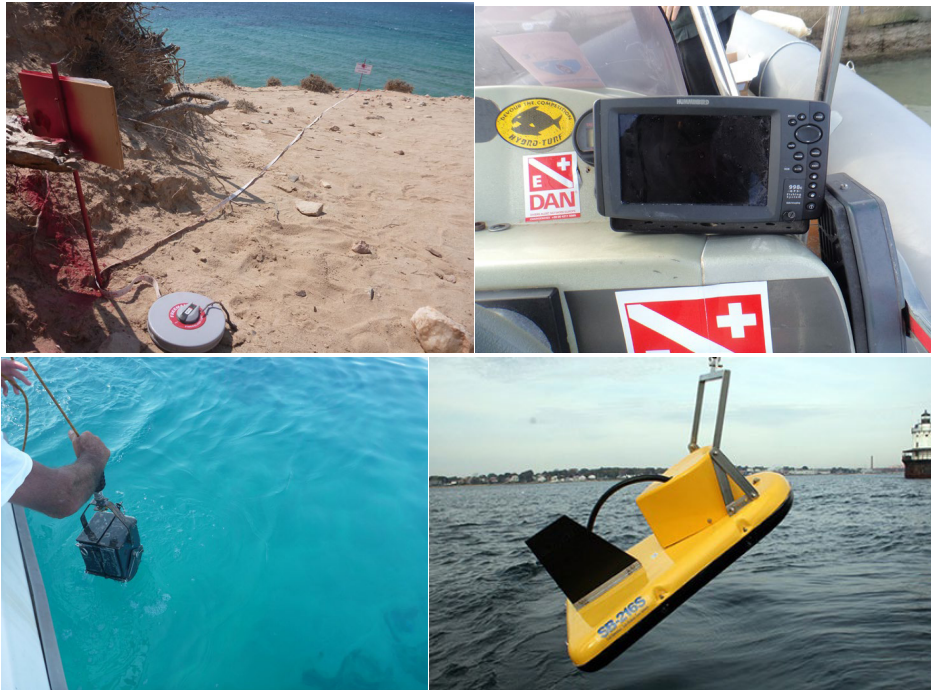
Fig. 30: a. Topographic sections, b. Side scan sonar, c. Sand samples, d. Sub bottom profiler. Photos by Alexandros Petropoulos.
