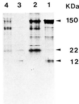
Fig. 3. Native polyacrylamide gel-electrophoresis of fractions from the FPLC-G 200 separation from root hairs and roots of *Glycine max* cv. Maple Arrow. 10 µg protein per lane. Lane 1: root hair, fraction 2; lane 2: root, fraction 2; lane 3: root hair, fraction 3; lane 4: root, fraction 3. Molecular weight marker proteins were trypsin inhibitor, ovalbumin and bovine albumin.
