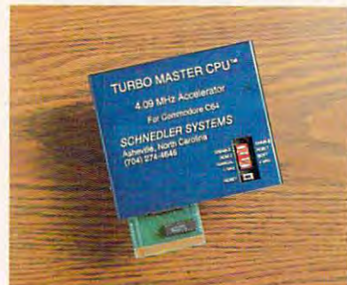
Boost your 64's speed to 4 MHz with the Turbo Master CPU accelerator.
