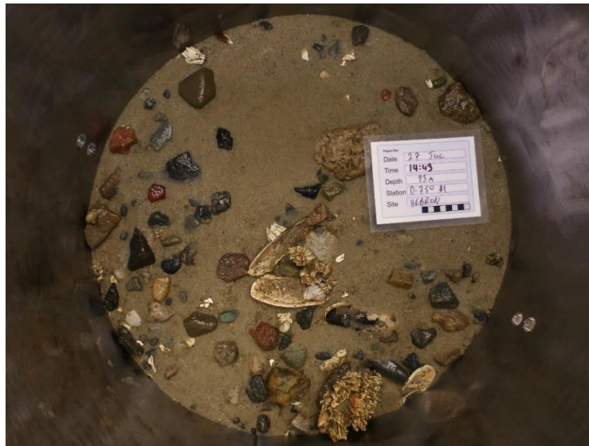
Figure 4-2 Example photo of sediment recovery with large volume box corer.
