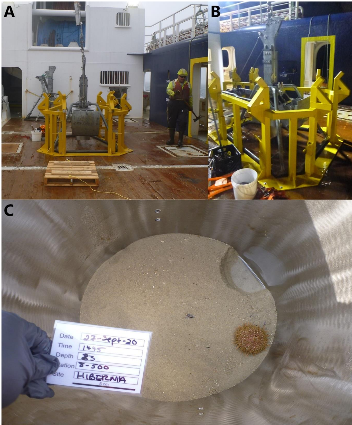
Figure 4-2: A) Deck operations of box corer in the cradle, B) Pouliot box corer closeup, C) Example photo of sediment recovered with the box corer.
