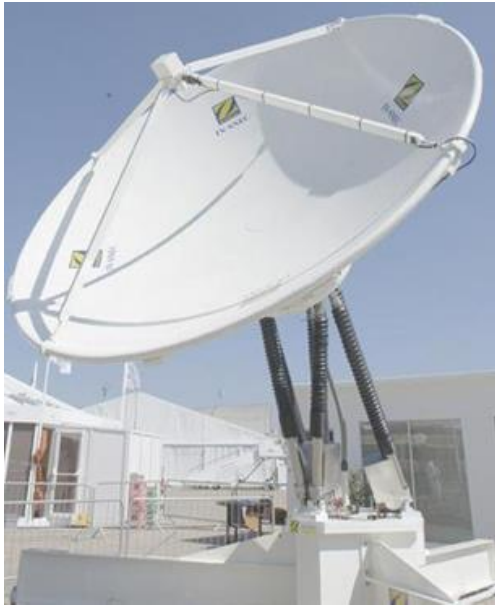
Figure 2-8: SANSА (1,2,3) This is a typical 6m antenna with a height of up to 12m.
