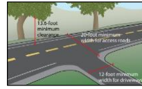
Figure 52. Road dimensions for emergency vehicles. (FEMA, 2008a).
