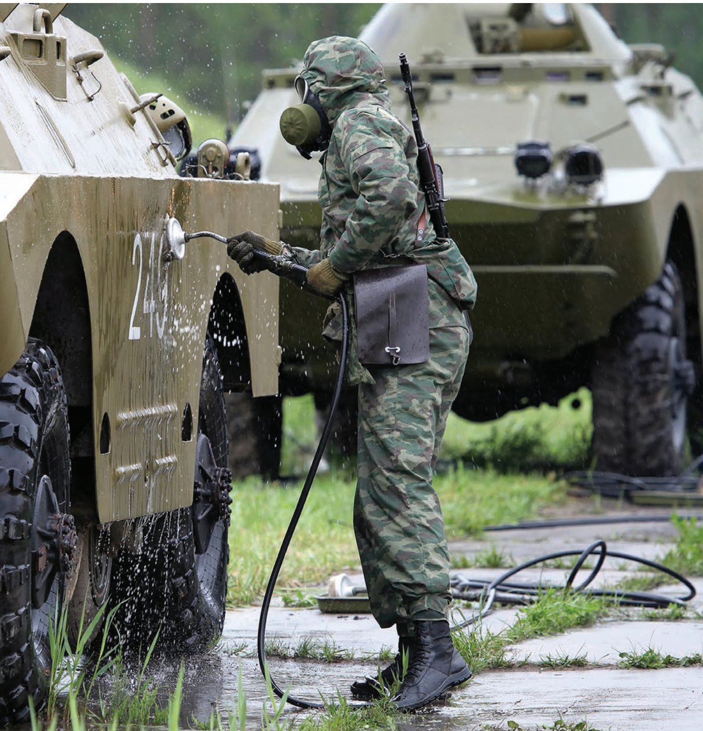
Pictured is a soldier of the Russian NBC troops decontaminating a vehicle with a ARS-14KM decontamination and degassing station. Photo: Vitaly V. Kuzmin, http://www.vitalykuzmin.net , Creative Commons Attribution-Share Alike 4.0 International license, Wikimedia
