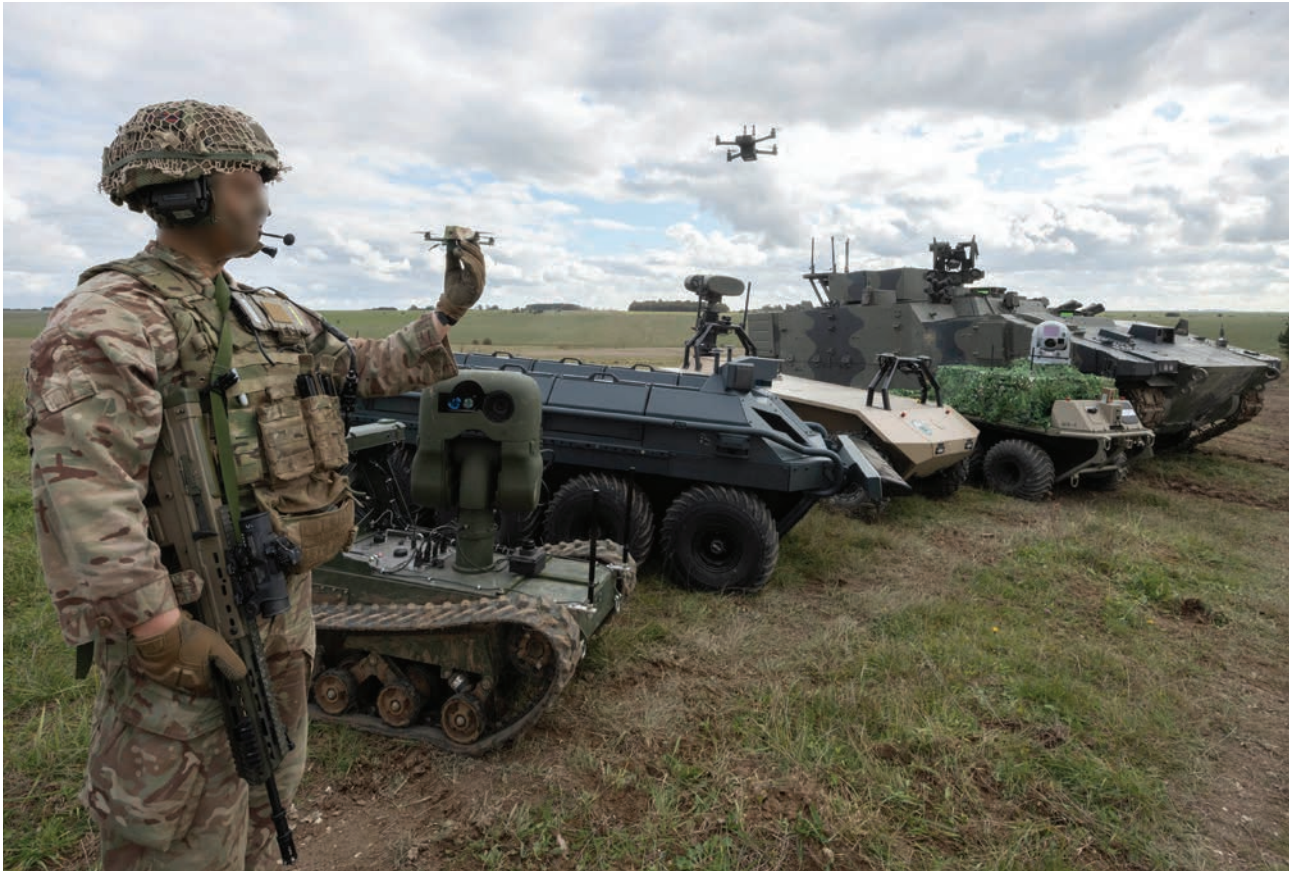
A selection of equipment on display at the Army Warfare Experiment (AWE) 2020. Left to Right: A soldier from 5 Rifles holding a Bug Nano UAV, an X2 unmanned ground vehicle, Mission Master unmanned ground vehicle, Viking unmanned ground vehicle, MUTT unmanned ground vehicle, Athena Armoured Vehicle. Photo: Sergeant Tom Evans, Crown Copyright
