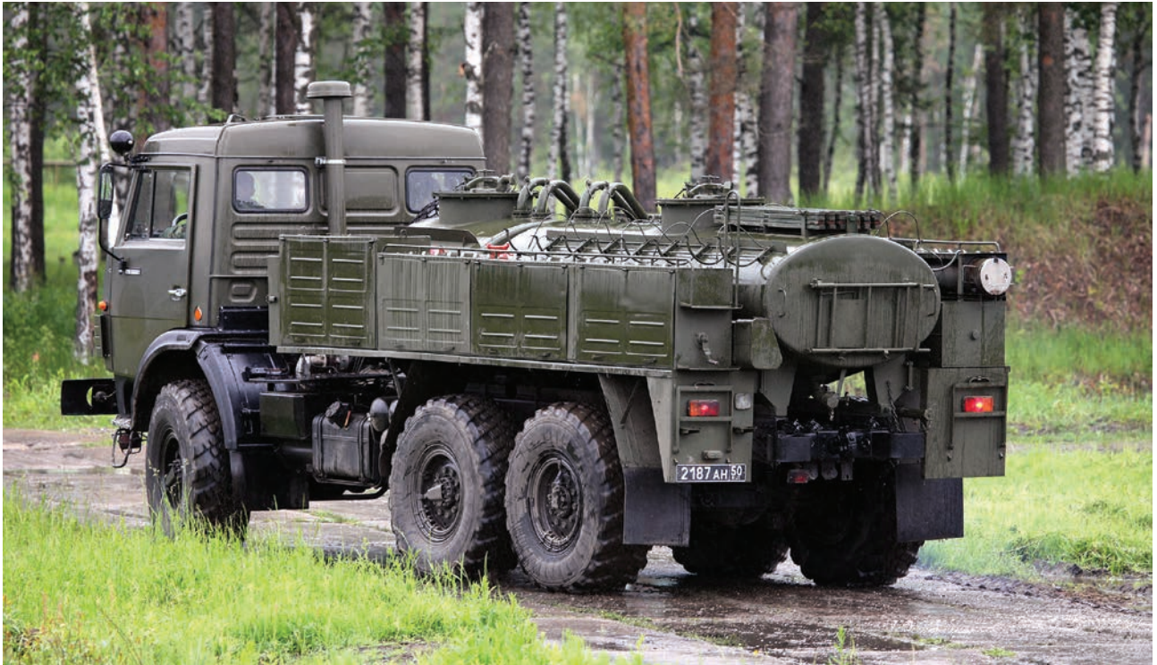
Pictured is a Russian ARS-14KM decontamination vehicle at the NBC Training Centre. Photo: Vitaly V. Kuzmin, http://vitalykuzmin.net , Creative Commons Attribution-Share Alike 4.0 International License, Wikimedia
