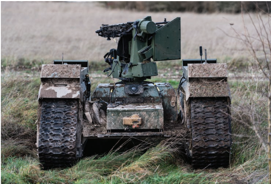
Pictured is the QinetiQ Titan Strike, a large tracked UGV with a laser rangefinder system during Army Warfighting Experiment, Autonomous Warrior 18. It is fitted with a machine gun –the weapon is under 100% human control remote operated. Photo: Corporal Rebecca Brown, Crown Copyright
