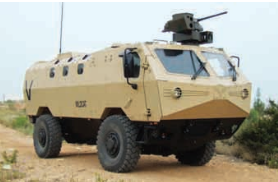
Based upon the high mobility Tatra oscillating arms 4x4 chassis, the Wildcat is an APC that can carry three crew members plus nine dismounts, at 18.5 tonnes GVW. (IMI)
