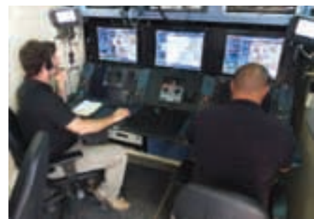
A definite boon for operators that already operate the Hermes 450 and who wish to either upgrade to Hermes 900 or operate both is that all ground control, datalink and C4I equipment remain the same. As can be seen here, it employs “glass cockpit” and hotas controls. (Armada/Eric H. Biass)
