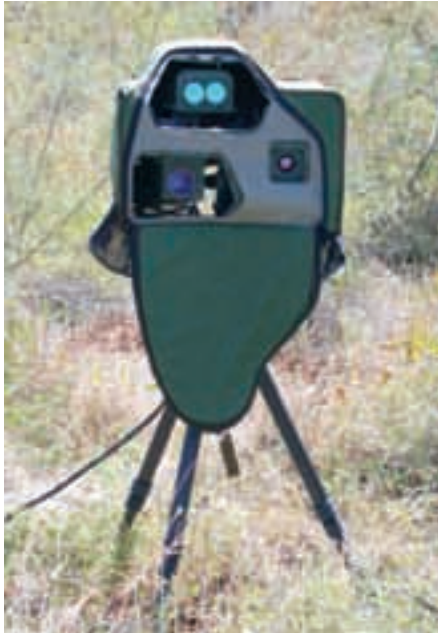
For the protection of infantry positions Rafael has developed a tripod-mounted version of its SpotLite gunshot detection. (Rafael)
