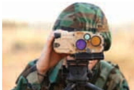
The Rattler-G (left) is one of the lightest laser marker/designators available; originally issued only to very specialised personnel, such as JTACS, this type of system is now issued to a wider audience. Very light, easy to use thanks to its shape, the Rattler H can designate a target for third parties up to a range of 3 km. (Elbit)
