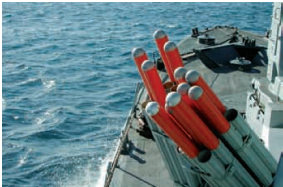
The Wizard geometrical shape decoy developed by Rafael is launched by the standard 115 mm launcher. (Rafael)
