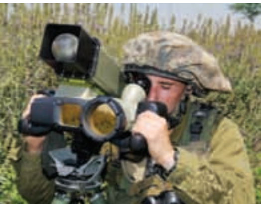
The Mini Spike features a radio link to the launch unit. It can be launched either from its launch unit or from the standard Spike infantry launchers. (Rafael)
