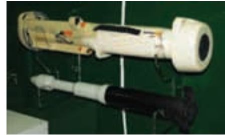
Developed by Israel Military Industries, the Shipon warhead is based on the follow-through-grenade concept. (Armada/P. Valpolini)
