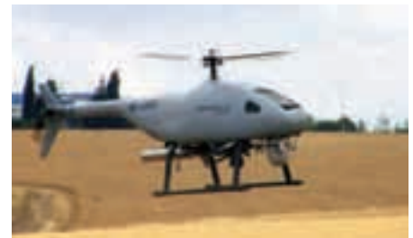
The Black Eagle 50's data link is from Elbit while typical payloads come from Controp, in this instance a D Stamp. (Steadicopter)
