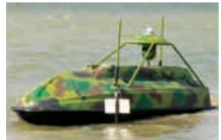
The ski-jet based Barracuda being developed by Top I Vision is able to hide low in reed marshes for a week. (Top I Vision)
