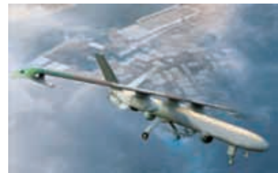
The now 550-kilo Hermes 450 has a payload capacity of around 180 kilos. Its ceiling is 18,000 feet and it offers an endurance of 17 hours. This artist impression shows it carrying electronic warfare gear in its underwing pods. (Elbit)
