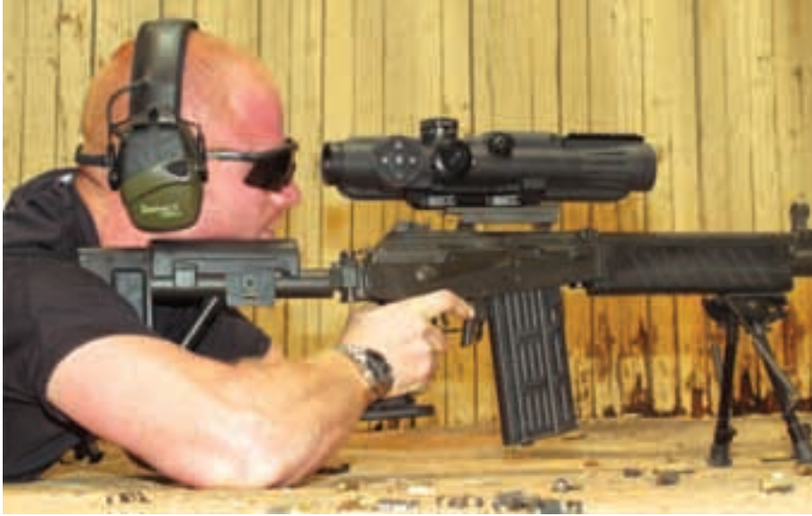
Meprolight Meslas includes a computer and a laser rangefinder, the sight thus providing the firing equation to the shooter. (Armada/P. Valpolini)
