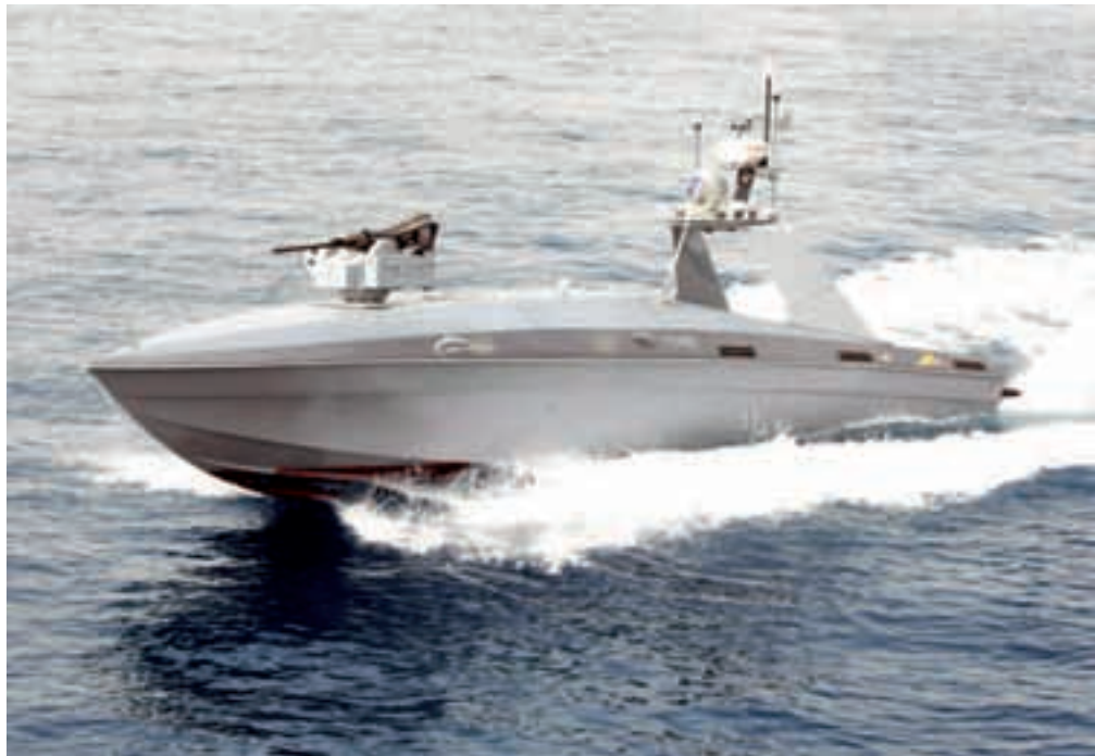
Elbit System's Silver Marlin is over 10 meters long and can be armed with a 12.7 mm RCWS for offensive operations. (Elbit Systems)
