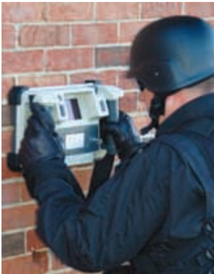
Camero's Xaver 400 is the mid-size see-through-the-wall radar developed by the company and is intended both for military and paramilitary use. (Camero)
