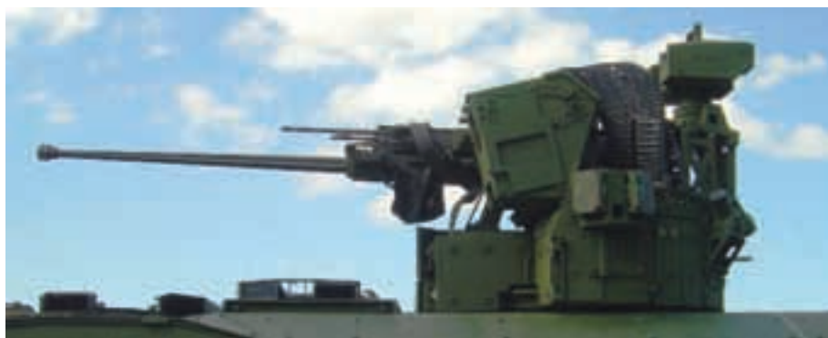
Elbit Systems UT30 unmanned turret; one of the last contracts is that for Brazil, where the turret equips part of Iveco's VBTP-MR Guarani 6x6 vehicles. (Elbit)
