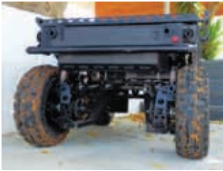
A four-wheel drive, four independent wheel suspension, four-steered wheel vehicle, the Lahav Rex is 160 cm long, 80 cm wide and 75 cm tall, and drives at a speed of 12km/hour. (Eric H. Biass)
