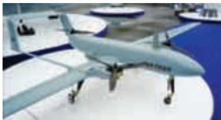
Here seen presented at the Paris Air Show in 2011 by IAI, the treble rotor Panther constitutes an innovative approach to convertible vertical-horizontal flight. It flies at an astonishing height of 5,000 feet above ground level. (Armada/Eric H. Biass)
