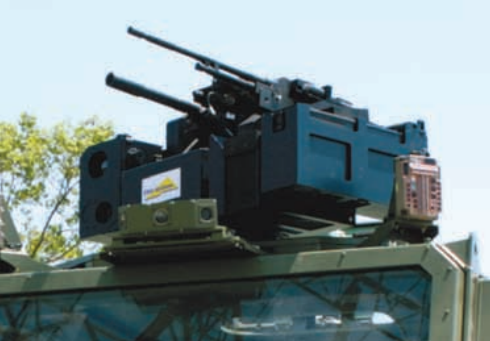
Elbit's Dual Remote Weapon Station can host a 12.7 mm or a 40 mm AGL in the main cradle and a 7.62 mm MG in the secondary one. (Elbit)
