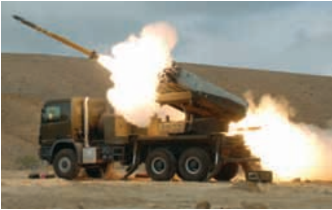
The Accular GPS-guided rocket (left) has a CEP of about 10 metres and a maximum range of 40 km. Israel Military Industries Extended Range Artillery Rocket (Extra) has an inertial/GPS guidance system and a range of 250 km. (IMI)
