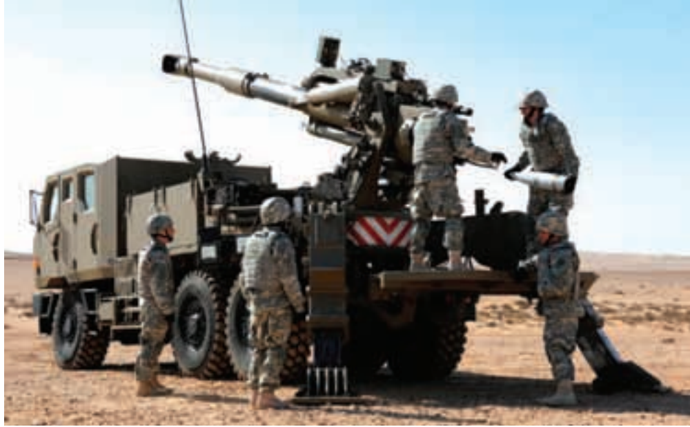
An ATMOS 155 mm truck mounted howitzer in action; a five-man crew ensures full operational capability to the system. (Elbit Systems)
