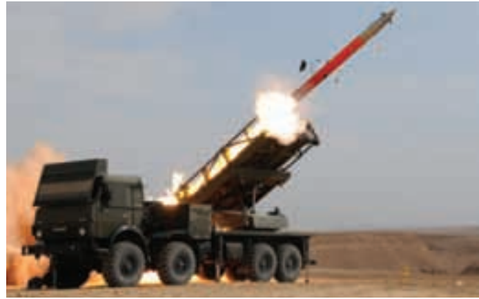
The Accular GPS-guided rocket (left) has a CEP of about 10 metres and a maximum range of 40 km. Israel Military Industries Extended Range Artillery Rocket (Extra) has an inertial/GPS guidance system and a range of 250 km. (IMI)
