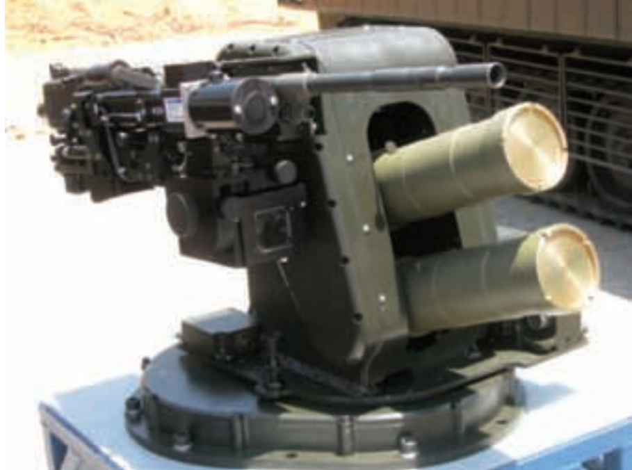
The Bright Arrow combines a remotely controlled weapon station and the hard kill element of the Iron Fist. (IMI)
