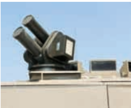
IMI defines the Iron Fist a second generation active protection system; it is made of a soft kill and a hard kill element. (IMI)
