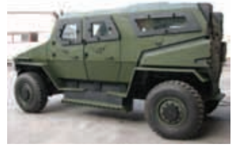
The 9.6-tonne Hurricane is currently being put in production on Hatehof assembly lines; it can transport up to seven people. (Hatehof)
