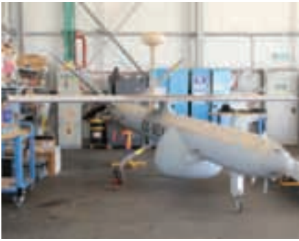
The evolution of the Hermes 450 never seems to stop as exemplified by this “guinea pig” photographed at the Pik airfield workshop in the Golan Heights, fitted with a new rotary piston engine, a three-blade propeller and an experimental radar gondola housing a Selex Gabbiano T20 maritime radar. (Armada/Eric H. Biass)
