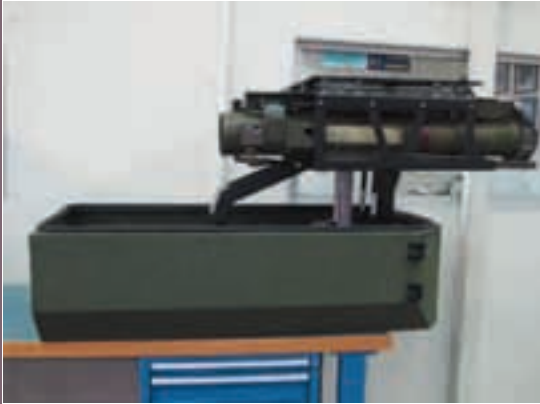
The new pod containing two Spike antitank missiles that can be retracted when not in use. It is aimed at the Samson MkI and MkII turrets. (Armada/P. Valpolini)
