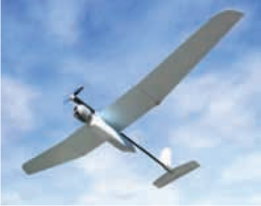
The electrically powered Skylark 1 LE weighs 7.7 Kilos, has an endurance of about three hours and lands by prancing into a deep stall at an adequate height above the ground and deploying a belly landing airbag. (Elbit)
