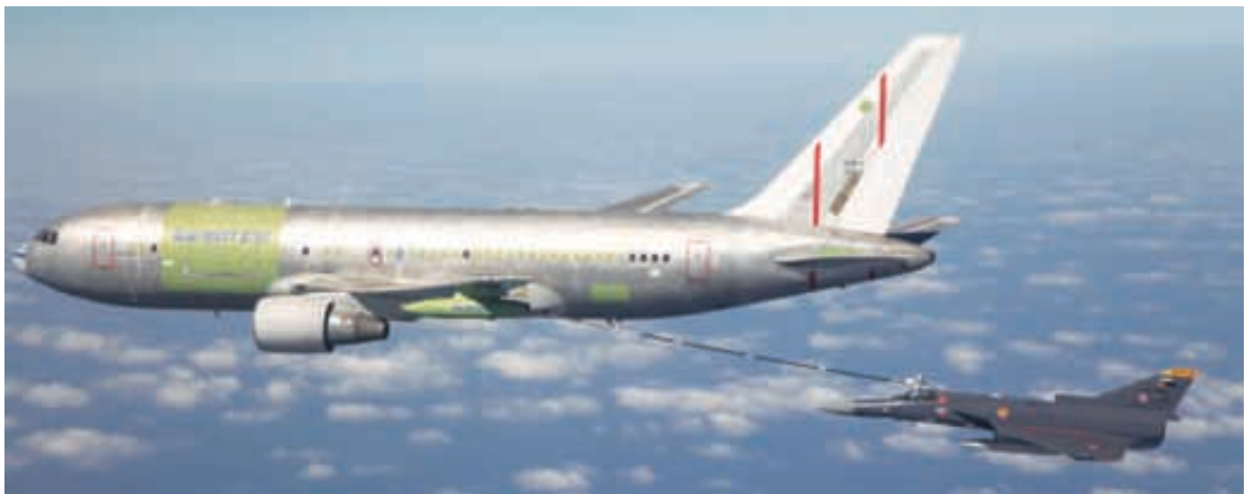
The first Colombian Air Force B767 Multi Mission Tanker Transport here seen test feeding a Colombian Kfir, is equipped with hose and drogue underwing pords. A second aircraft is expected, equipped with a fly-by-wire air-refuelling boom. (IAI Bedek)
