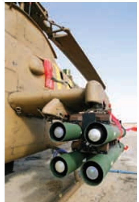
A Rafael Spike ER on a Cobra attack helicopter. This missile has also been integrated in the Eurocopter Tiger and in the AgustaWestland A129 Mangusta. (Rafael)
