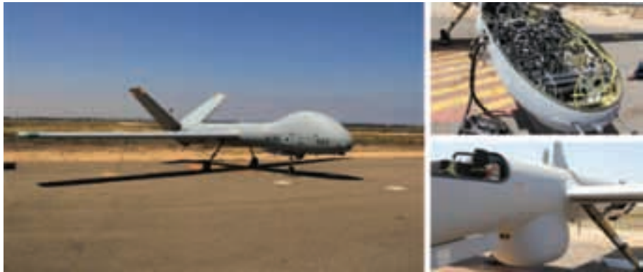
Photographed by the author at the Pik airfield in the Golan Heights, the 15-metre span Hermes 900s display their ample bays enabling them to carry an impressive array of sensors, including a maritime surveillance radar. (Armada/Eric H. Biass)
