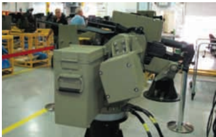
A Samsom Mini on the assembly line at Rafael main plant in Haifa (left). The type has been selected by Israel for its Namer and by undisclosed export customers. One of Rafael best sellers in the turret field, the Samson Mini (right), can be armed with weapons up to 12.7 mm machine guns or 40 mm AGLs. (Armada/P. Valpolini)
