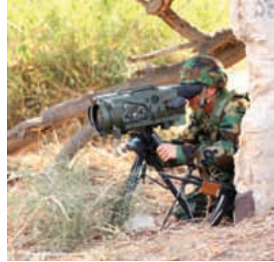
Elbit's Long View CR allows one to recognise a man at 7 km distance, thanks to its x18 zoom. (Elbit)
