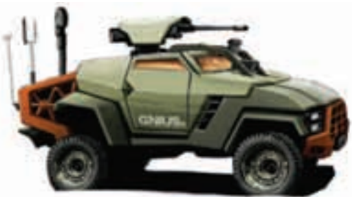
The projected G-nius Guardium Mk.III robotic vehicle would be based on a Ford truck and would carry a Rafael turret. (G-nius)
