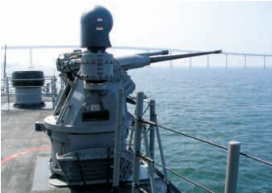
The Typhoon accommodates weapons up to 30 mm. This example is installed on a US Navy ship and is equipped with a top optronic sight. (Rafael)
