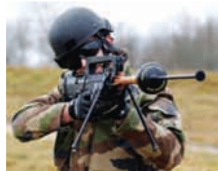
A light system for ramming doors open, the Simon rifle grenade developed by Rafael is one of the numerous breaching systems born out of the IDF experience. (Rafael)
