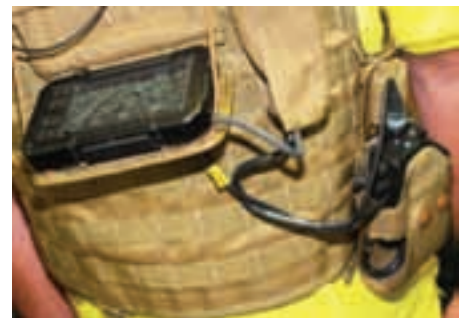
The Dominator LD 4.3-inch display (left) and Raptor terminal linked to the soldier radio. The system developed for dismounted soldiers weighs only 1.3 kg. (Armada/P. Valpolini)
