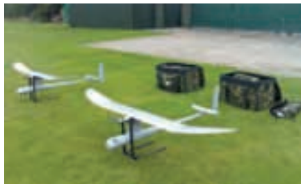
The electrically powered Top I Vision Casper 250 comes in a neat compact package that includes aircraft, datalink aerial and control station. (Top I Vision)
