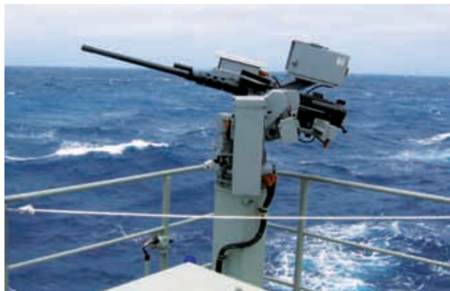
A Rafael Mini Typhoon remotely controlled gun mount armed with a 12.7 mm machine gun. It has a maximum weight of 170 kg. (Rafael)
