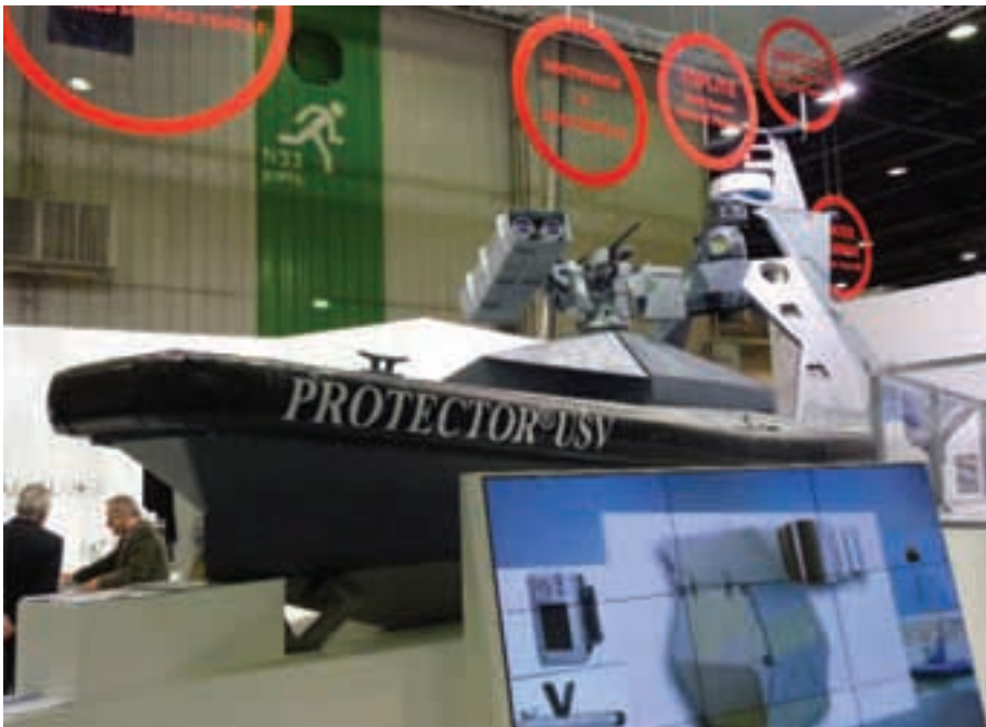
The new Rafael Protector 11, here photographed at the 2012 Euronaval exhibition in Paris, is impressive and comes, from left to right, with a Spike twin launcher canister attached to a Typhoon gun turret, loudspeakers, a Toplite electro-optical turret, two multiple 180° camera systems (the second unit looking rearwards), a detection radar, and finally a powerful water cannon mounted on the rear platform. (Armada/Eric H. Biass)
