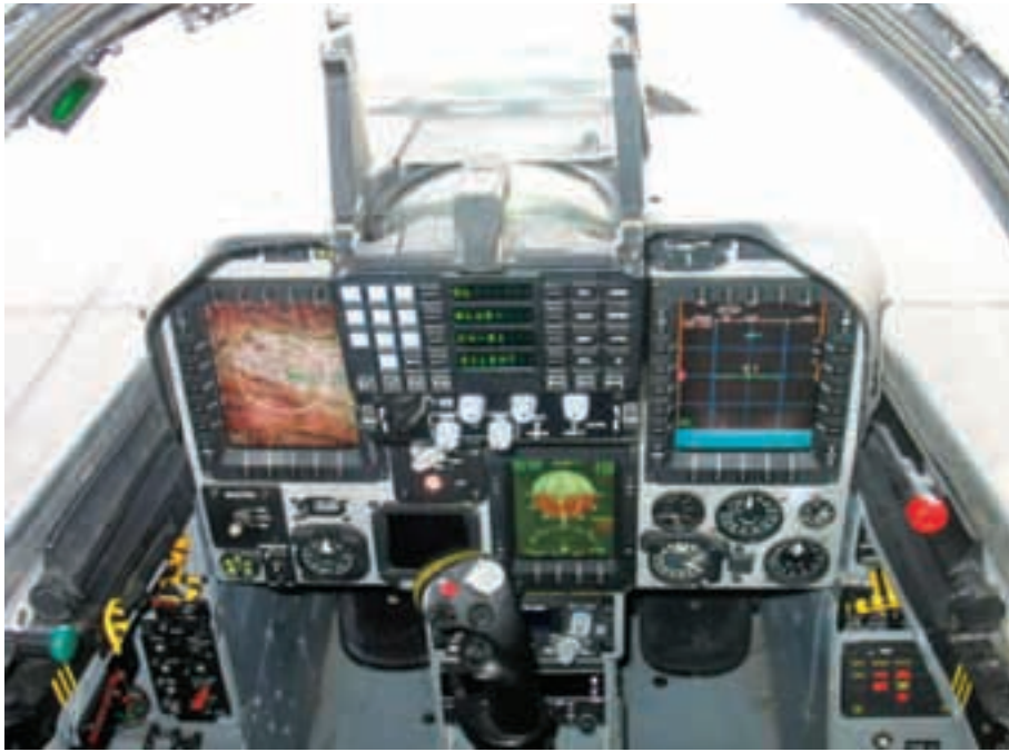
The Kfir Block 60's cockpit, complete with multiple function display, mapping display, flight computer and modern head-up display. (IAI)
