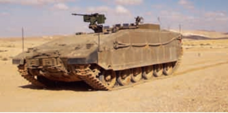
Derived from the Merkava MBT the Namer is one of the heaviest armoured personnel carriers in the world. For the future Israel is looking at a lighter vehicle family. (Rafael)
