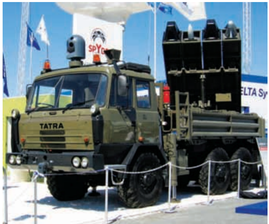
Displayed at the 2005 Paris Air Show, the Spyder illustrates Rafael's involvement in shore-based systems, by using existing air-launched missiles like the Derby (left) and the Python. (Armada/Eric H. Biass)
