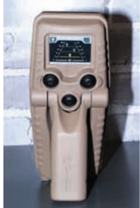
A view of the latest version of the Xaver 100 sporting a screen that displays the symbols of human beings and their distance from the wall. (Armada/P. Valpolini)
