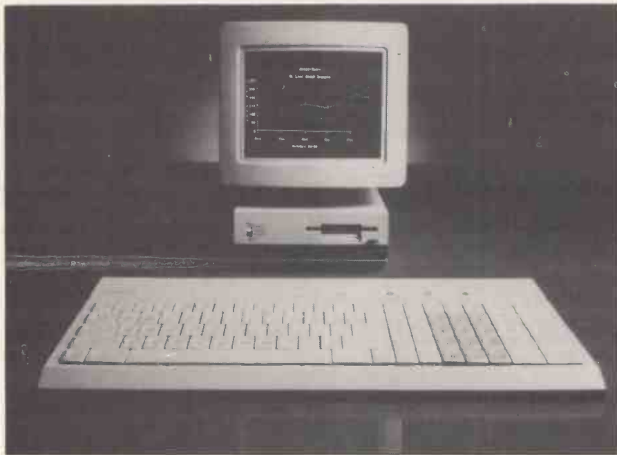
The F1 keyboard has to be positioned precisely to maintain its infrared link.
