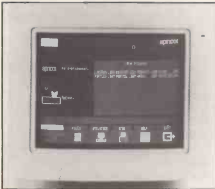
The opening menu with its command window. Icons are displayed along the foot of the screen.
