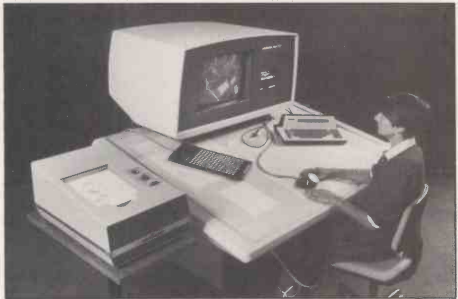
The Gradis 2000, with the operator holding the cursor which is used for digitising.
