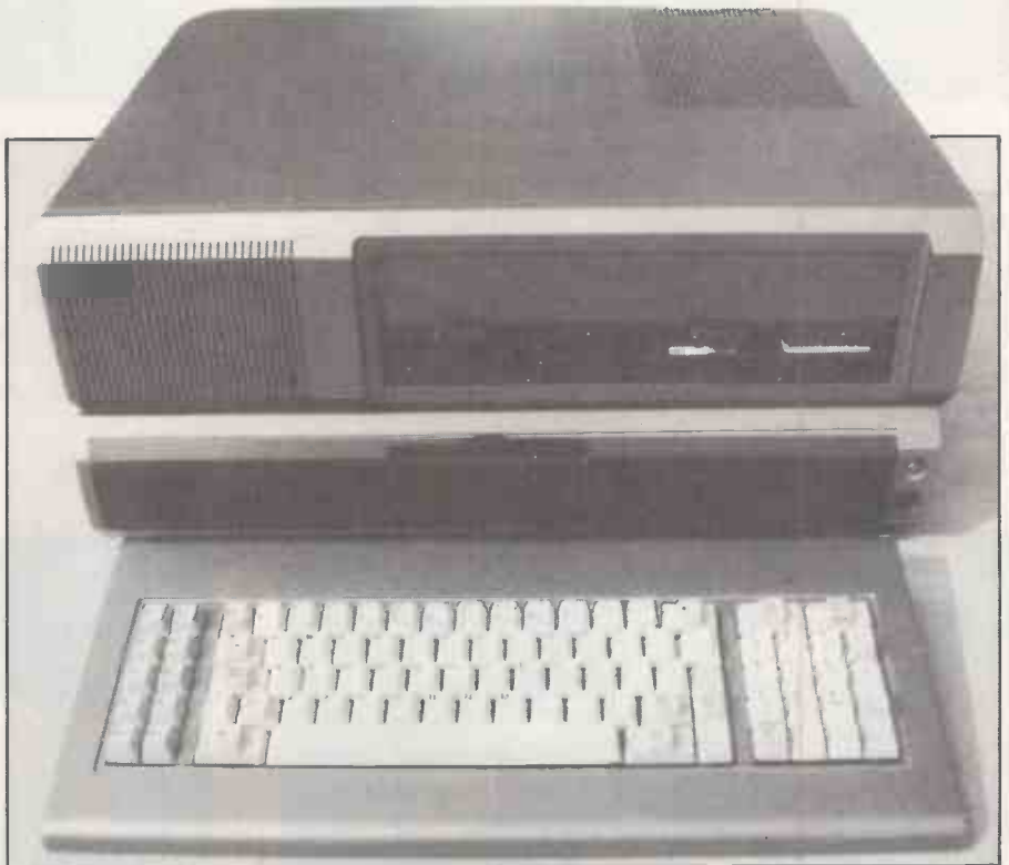
There is no separate Model B, an expansion unit converts the Model A into a Model B.
