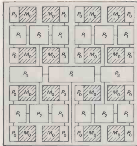
Figure 5. Lay-out for a binary processor tree.
