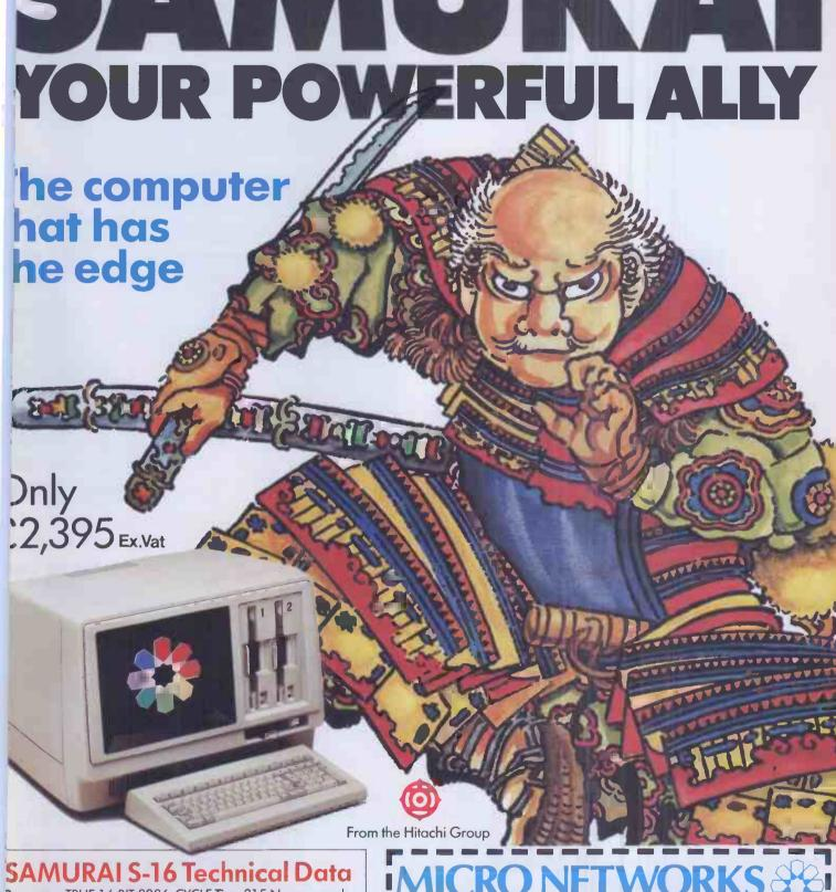
Processor: TRUE 16-BIT 8086, CYCLE Time 215 Nano seconds. Co-Processors (optional): 8085, 8087. Architecture: DMA Bus Based. Speed: DMA @ 6.4 MB/SEC; DISC transfer @ 3MB/ SEC. Memory (RAM): 128KB Standard, expandable to 640KB. Screen: High resolution green: anti-glare optical filter; colour and graphics optional. **DISCS**: Two 8" DS/DD giving 2.36 MB formatted IBM compatible: Hard DISC optional. Interfaces: 2 RS 232 Communications interfaces. Plus: Centronic printer interface
