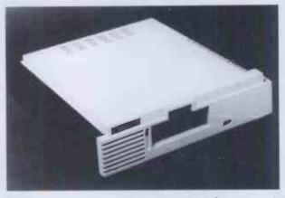
A Multi-User System, using a Hard Disk System as the Hub Processor, and operating under McNos a proven CP/M\* Compatible Operating System, up to 16 users are available, each User Workstation has 64KB and its own Processor to provide full speed operation.
