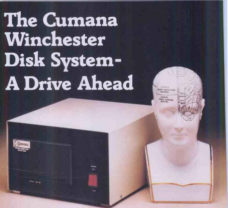
Cumana's top quality 51/4 inch Winchester hard disk drive gives TRS-80 model III/IV users high capacity at low cost, with formatted storage capacities from 5.25 to 21.00 MB.
