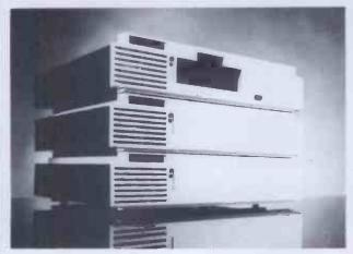
A Flexible Disc System, Z80A based, CP/M\* Operating system, 400KB, 800KB, or 1.6KB storage on twin  $5\,\%$  diskettes.
