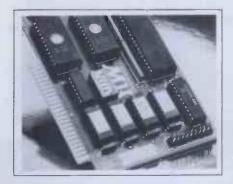
FOR APPLE II COMPUTERS, Microbuffer II features on-board firmware for text formatting and advanced graphics dump routines. Both serial and parallel versions have a power-efficient low-consumption design. Special functions include Basic listing formatter, self-test, buffer zap, and transparent and maintain modes. The 16K model is priced at \$259 and the 32K, at \$299.
