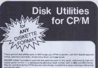
DTEST tests a disk for bad spots. Bad sectors are locked out from later use by CP/M by automatically collecting them in a -garbage+ file. All errors are reported to printer and/or console, Reduces probability of later disk crashes. Indispensible for hard disks, as media cannot be replaced. Use DTEST before disk errors ruin your work!
