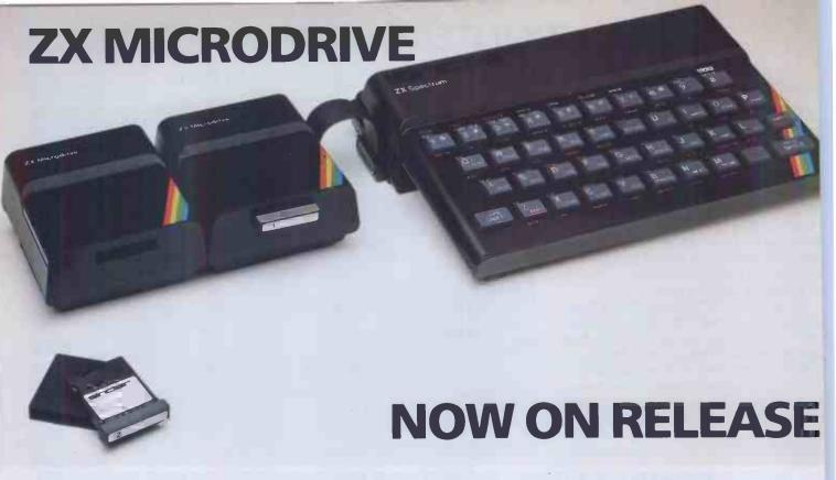
The ZX Microdrive System – as you'd expect from Sinclair – is unique to the world of computing. It's a compact, expandable add-on system which provides high-speed access to massive data storage. With just one Microdrive alone (and Interface 1), you'll have at least 85K bytes of storage, the ability to LOAD and SAVE in mere seconds, the beginnings of a local area network of up to 64 Spectrums, and a built-in RS232 interface! The cost? Less than £50 for each Microdrive.
