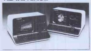
Integrated Desk Top Computer with 12 inch Bit-Mapped Graphics or Character Display, 64Kb RAM, 4 MHz 280A (© Two Quad Capacity Floppy Disk Drives, Selectric\* Style 87 Key Keyboard, Business Graphics Software.
