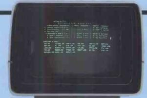
A VDT-6—12" high resolution, green phosphor CRT with a 24 x 80 character display and detachable keyboard.
