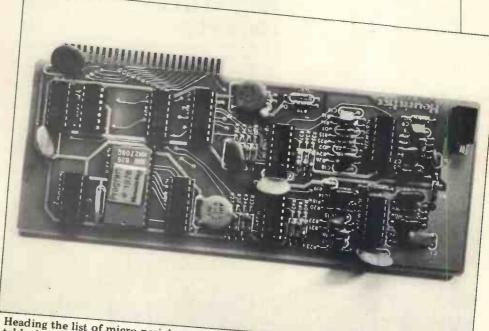
Heading the list of micro-peripheral exotica, the SpeechLab can offer an acceptable degree of voice command recognition.
