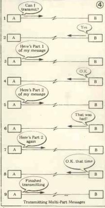
the error rate encountered on dial-up lines might be too great to transmit messages of more than about 80 bytes reliably. Even at shorter lengths, re-transmissions will be necessary. These should be counted as a means of moni-toring line quality. When things get really bad you will find that you have to re-transmit your retransmissions! This is usually time to quit and dial a new circuit.
