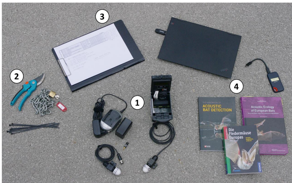
Figure 24: Sampling material for bat survey: 1. Bat logger including microphone, batteries and sd card; 2. Safety chains for the logger and strings to install and direct the microphone; 3. Field sheet to write the survey date and other important notes such as the bat logger code 4. Computer, software, hard disk, and books to identify and store bat calls.
