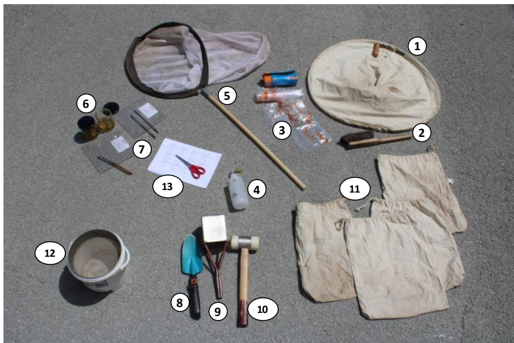
Figure 32: Sampling material for invertebrate sampling: 1. Beating net; 2. Hand broom for beating on branches and collecting the animals in the collection tube; 3. Plastic bags; 4. 75% ethanol; 5. Sweeping net; 6. Pitfall trap (glass jar filled with 200 ml propylene glycol); 7. Polycarbonate Lexan® roof with threaded metal bars; 8. Small spade; 9. Soil stamp; 10. Sledgehammer; 11. Linen bag; 12. Bucket with 2mm sieve; 13. Labels.
