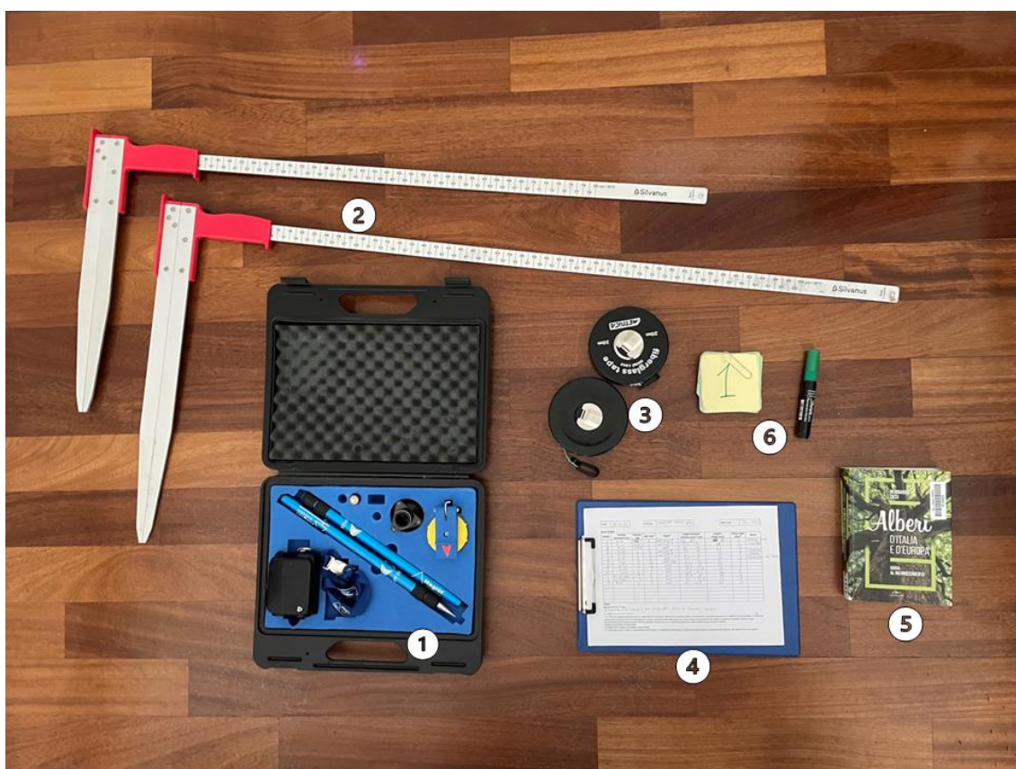
Figure 41: Essential material for fieldwork: 1) Vertex and its accessories; 2) Forest callipers; 3) Measuring tapes; 4) Field data sheets (with writing tablet); 5) Tree species manual; 6) Post-its and various stationery material (pens, markers).
