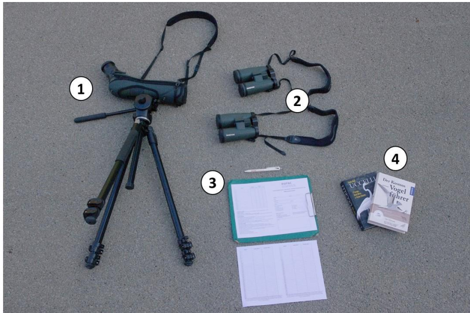
Figure 20: Sampling material for the bird survey: 1. Telescope for identifications beyond a 100-meter distance with 25 to 50 magnification; 2. Two binoculars with a resolution of 10×42 and 8×42; 3. Datasheets and pen for data collection and site conditions; 4. Field guide for bird identification, mainly for intern training.
