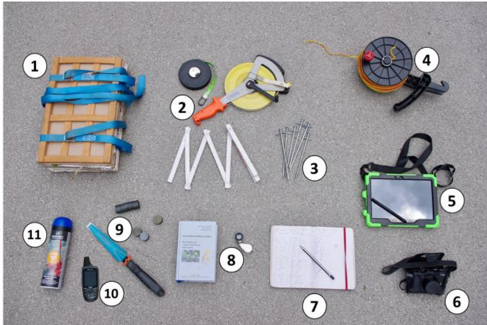
Figure 14: Sampling material for the botanical survey: 1. Plant press for herbarium specimens; 2. 2 m folding ruler, 10 m and 50 m measuring tape; 3. Tent pegs; 4. Reel with 150 m string for delimiting the forest plots 5. Tablet with GIS Software for habitat mapping; 6. Digital camera for photo documentation; 7. Field book and pen; 8. Folding lens and field guide for identifying species in the field; 9. Magnets and small spade; 10. Handheld GPS; 11. Color spray can for marking corner points.
