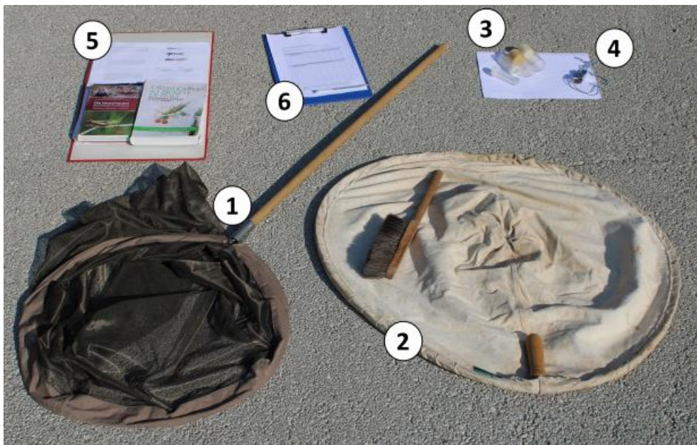
Figure 26: Sampling material for the grasshopper survey: 1. Sweep net; 2. Beat net; 3. Collecting recipients, empty and with ethanol; 4. Magnifying glass; 5. Literature for species identification; 6. Field sheet to write the survey data (Appendix 15.1).
