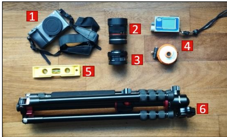
Figure 46: material for canopy photographs; 1: camera; 2: fisheye lens; 3: normal lens; 4: vertex and transponder; 5: level; 6: tripod.
