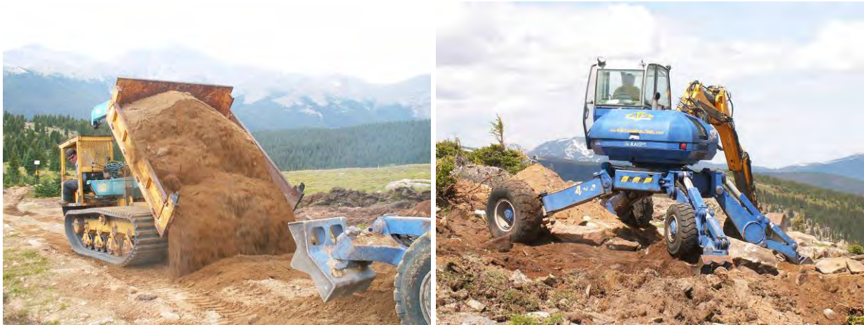
Photo: Maruka rubber tracked dump truck and spider hoe used on the Eagle Wind lift.
