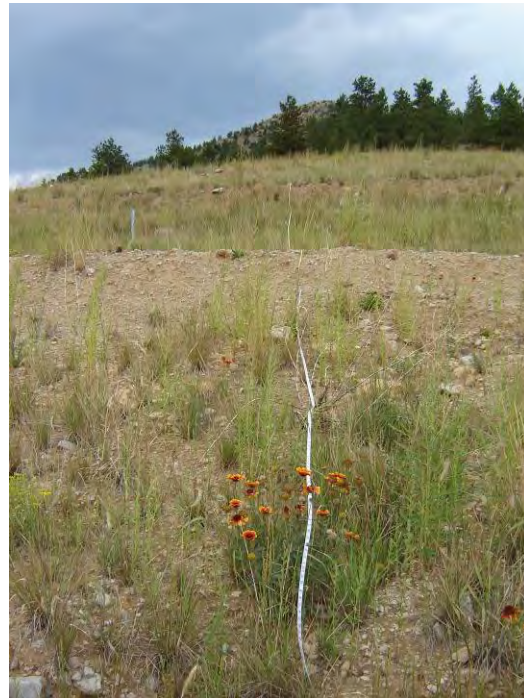
Photo 15. Sampling transect running up waste rock repository slope.
