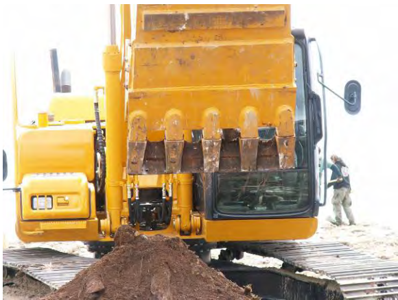
Photo: Welded bar for topsoil salvage spider hoe machine plant and topsoil salvage together
