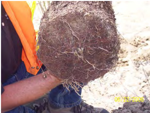
Figure 9 – Root development with 4:1 soil:bentonite mix
