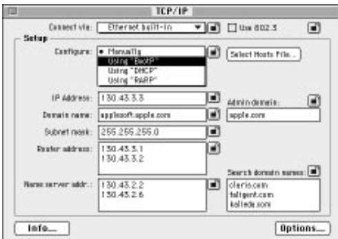
figure 2 / The new TCP/IP control panel's Administrator mode has advanced features, such as a more powerful domain-name resolver (lower right) that uses implicit and explicit search paths.
