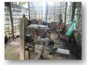
Fig 5.4.8 Rice huller integrated with IWME
