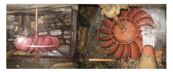
**Improved Water Mill:** This technology helps generate off-grid electricity for mountainous countries like Nepal, where there are plenty of water resources and there is a tradition of constructing water mills due to the geography of the region. The technology uses the energy of falling water, kinetic energy, which it converts first to mechanical, and then to electrical, energy. It is a valuable source of power for domestic use as well as for energy-using micro-enterprises.
