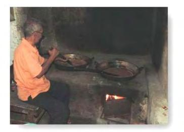
Fig 5.3.3 Rajapakse with his improved two-burner cookstove used for milk-coffee production
