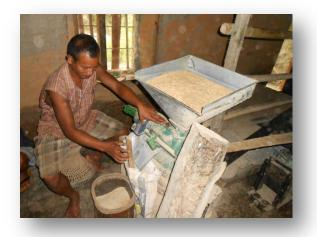
Fig 5.4.7 Paddy processing in rice huller
