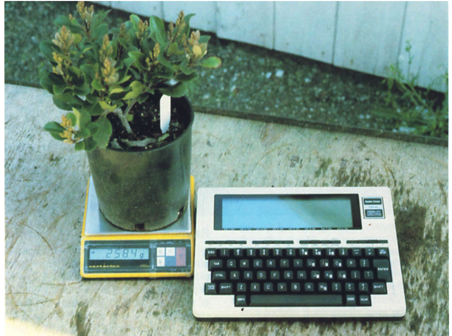
Water use, as measured by weight changes of plants in containers, was determined with a digital balance attached directly to a portable microcomputer.
