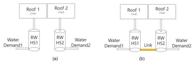
Figure 1: Schematic of rainwater harvesting system (RWHS); (a) two single RWHS; (b) connected RWHS
