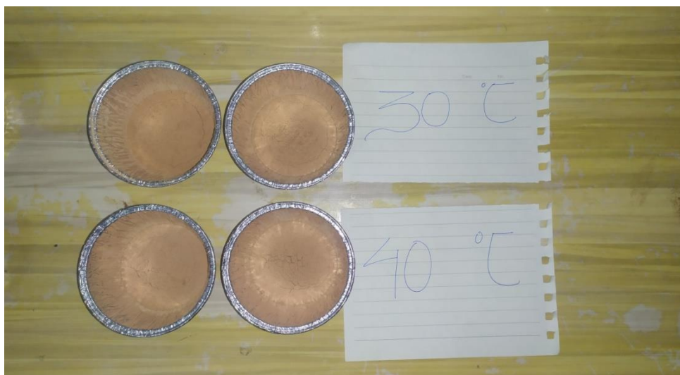
Figure 6-10. NaOH flour sample after oven.
