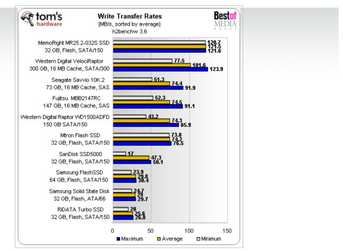
A write speed of 120 MB/s is a result that might have been stimulated by the Adaptec controller's cache memory. However, the data transfer diagram clearly shows that this drive maintains this high throughput.
