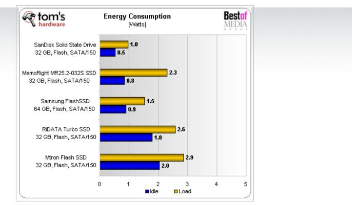
Memoright isn't only faster than Mtron, it also required less power. A power consumption of 0.8 W instead of 2.0 W when idle is an excellent result, which is comparable to fast conventional 2.5" hard drives. The maximum power requirement is also lower at 2.3 W. Conventional hard drives require up to 4 W.
