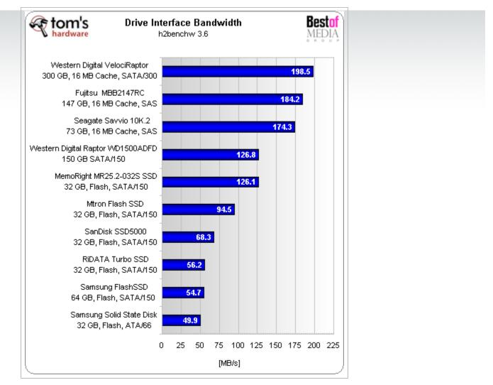
Interface performance reflects the maximum throughput for the Serial ATA interface. The Memoright's SATA interface supports 150MB/s operation and is limited to 126 MB/s, which equals the highest transfer rate to or from the flash memory chips. Other hard drives reach better interface throughput because they come with an additional cache memory (DRAM), which is even faster than Flash.
