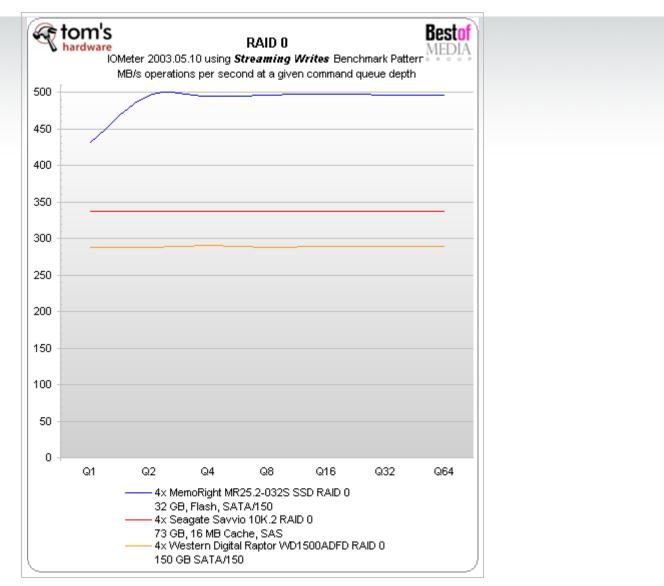
Streaming write performance is similar. It is important, though, to be aware that the controller cached most of the writing operations, hence the graph is somewhat inflated. The result of 430 MB/s at single commands (Q1) is realistic.
