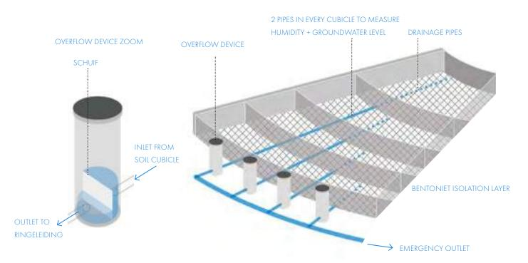
Scheme detail of the design for hydrological monitoring in the Soil cubicles.
