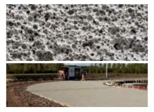
Porous concrete is a special type of concrete with a high porosity that allows water from precipitation to flow through it. Thereby it reduces runoff/drainage and allows groundwater to recharge. It is mainly used in parking areas with light traffic, residential streets, pedestrian paths and bike trails.
