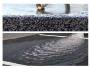
Porous asphalt pavements offer new tool for managing storm water. These pavements, used mostly for parking lots, allow water to drain through the surface into a stone recharge bed and infiltrate into the soil afterwards. The strength and resistance of porous asphalt pavements concerning traffic load, is claimed to be similar to conventional asphalt paving.
