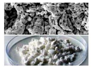
Upsalite is the most absorbent material discovered yet. The extraordinary properties of this new material were discovered by chance by a group of scientists in Uppsala (Sweden). The powerful absorbent capabilities are given by its three-dimensional structure with pore sizes of a nanometre(!), turning it into a stable and light material.
