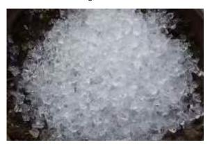
Superabsorbent polymers are artificially synthesized hydrogels with high water retention properties and high storage capacity for longer periods of time. There are many types of polymers and the most efficient ones are the biodegradable polymers based on cellulose, especially because they create small reservoirs of water to enhance water availability for plants. Upsalite
